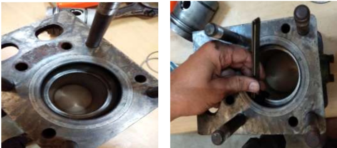
Plate 3.19 Gap Measurement by Feeler Gauge
