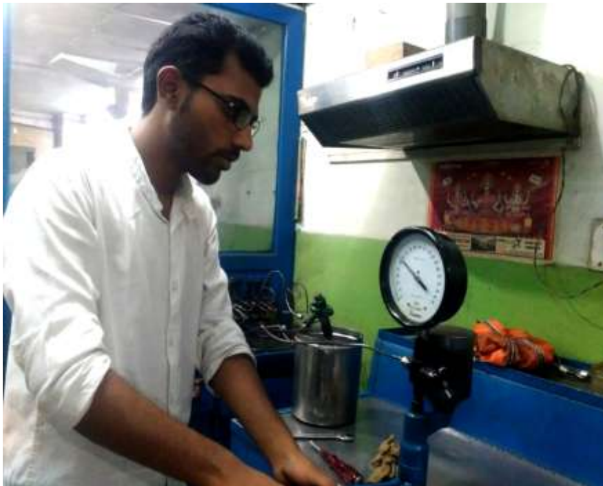
Plate 3.17 Fuel Injector Pressure Measurement
