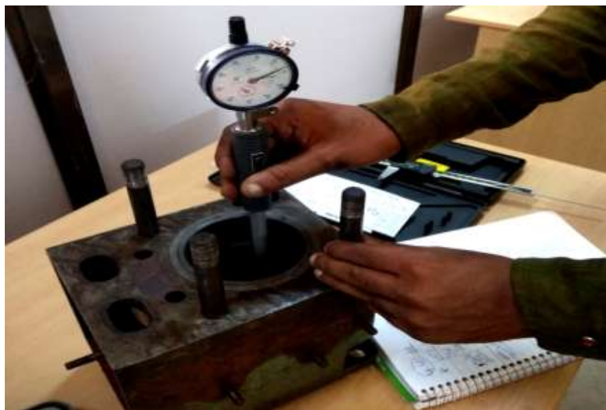
Plate 3.15 Cylinder Bore Measurement
