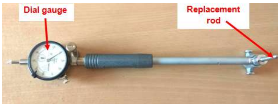
Plate 3.14 Cylinder Bore Gauge
