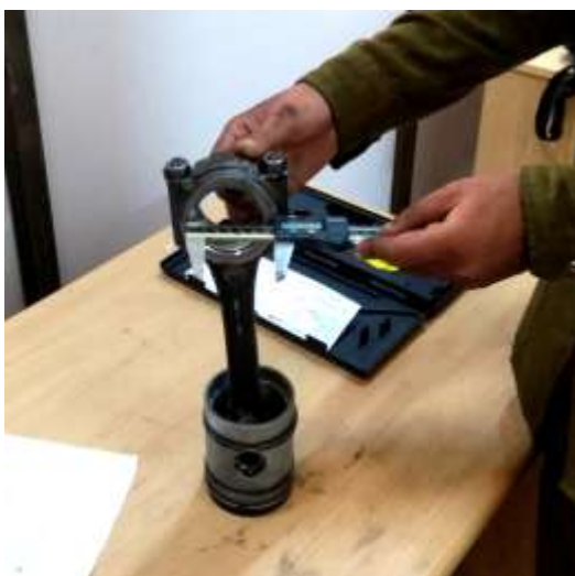
Plate 3.12 Measurement of Inside Diameter of Big End Bearing of Piston
