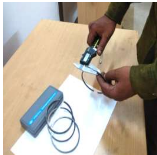
Plate 3.13 Measurements of Piston Ring and Oil Ring
