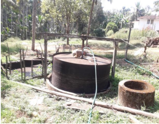
Plate 2: Floating drum type biogas model
