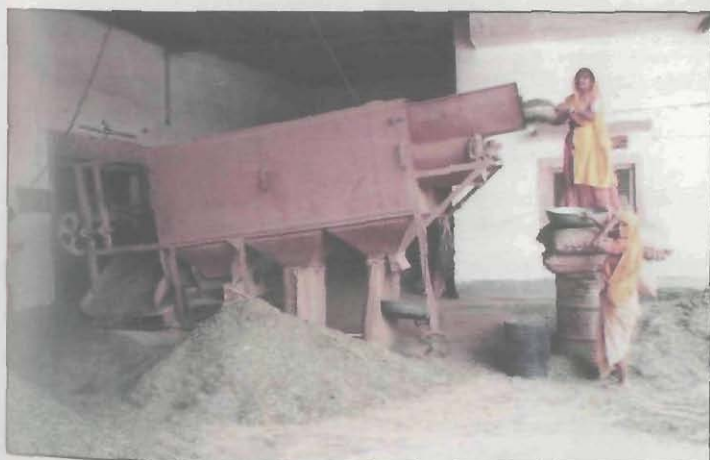
Fig. 6. Cleaning of henna leaves in a processing unit
