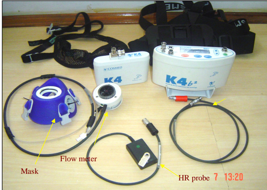
Fig. 3.13 Computerized Ambulatory Metabolic Measurement System (K4 b 2 ).
