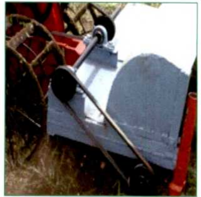
Power transmission from gear box
