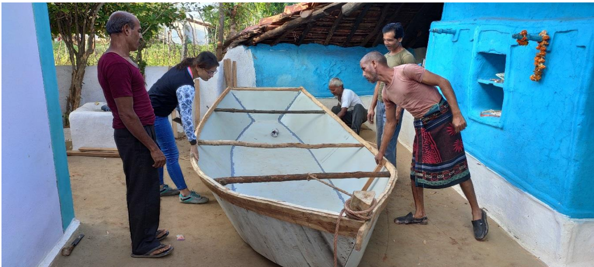
Plate 2: Wooden frame tin sheet boat manufactured by fishers
