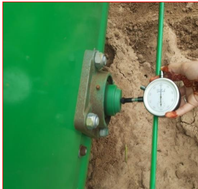
Plate 3.36 Measurement of rotor speed by Analog Type Tachometer
