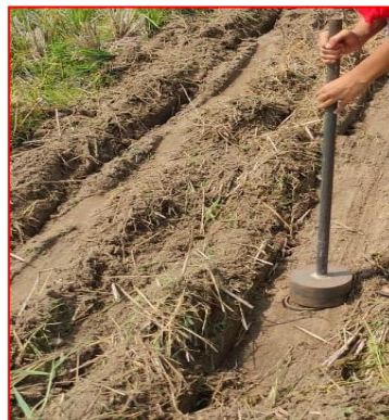
Plate 3.31 Determination of Bulk density by Core cutter method
