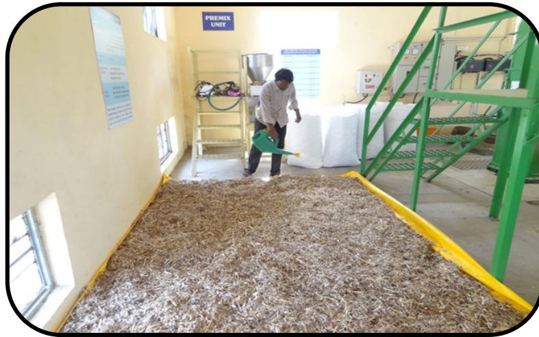
Spraying of enzyme solution on shredded cotton stalk with different dilution
