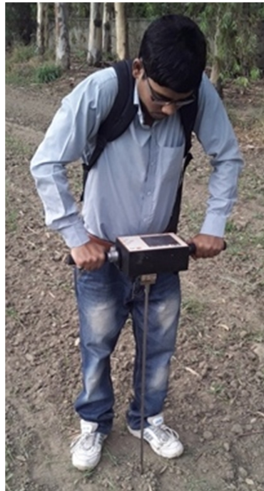
Fig 3.8 Soil hardness being measured using a digital cone penetrometer.
