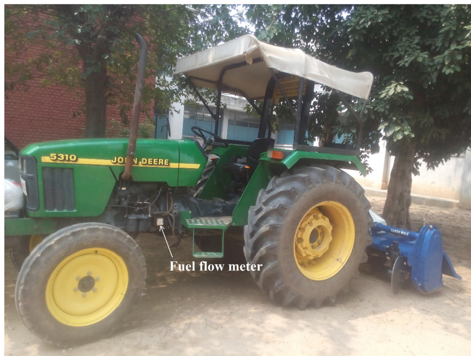
Fig 3.6 A view of tractor equipped with the fuel meter.
