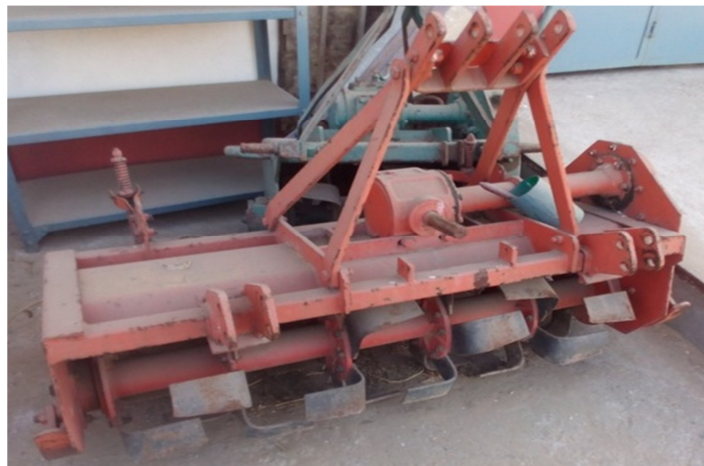
Fig 3.4 A stationary view of the rotavator with L type blades.
