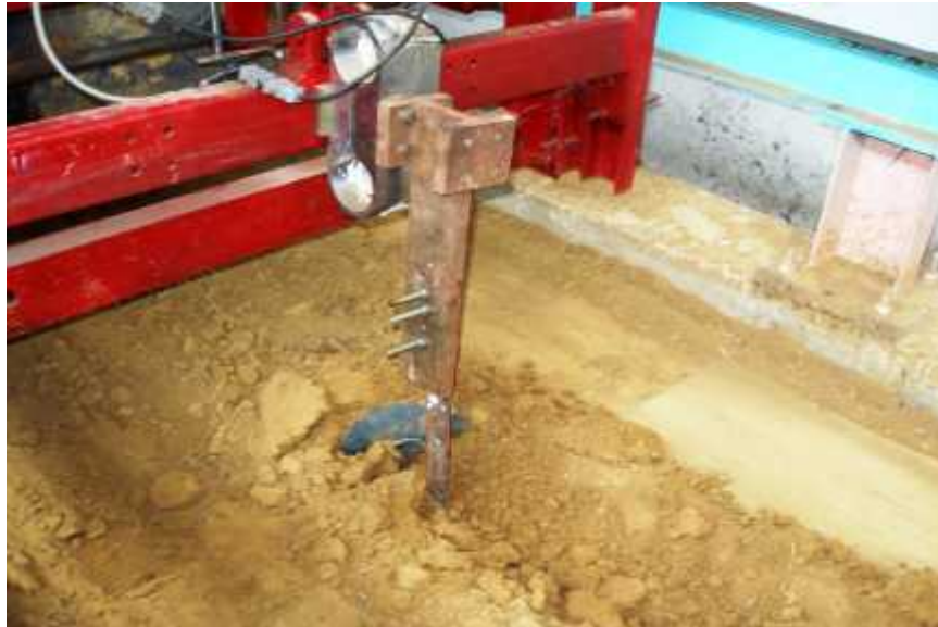
Fig 4.14 Test run of Plow for measurement of Draft
