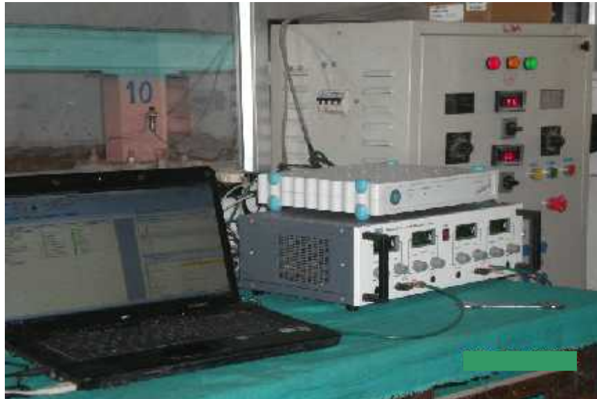
Fig 4.9 Data acquisition system & Lap top
