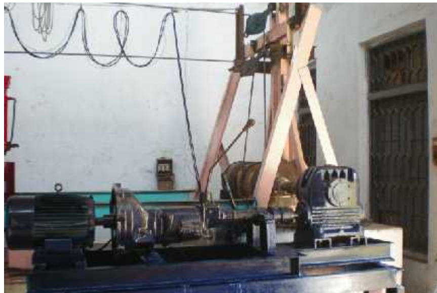
Fig. 4.8 Motor for drive of Processing Trolley and Test Trolley
