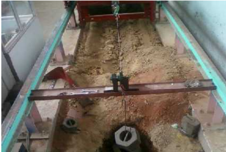
Fig.4.11 Pulley with bracket and Spring Dynamometer
