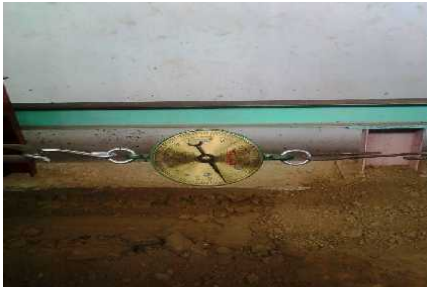
Fig.4.12 Spring Dynamometer used in calibration of EORT
