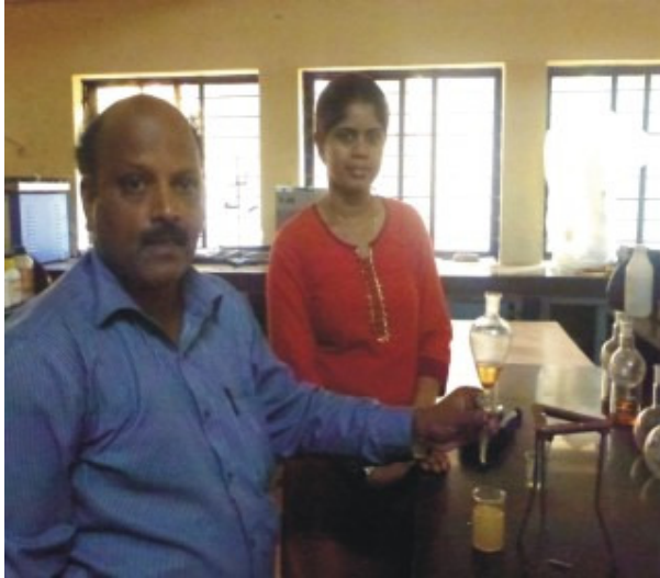
Plate 4b: Separation of biodiesel and glycerol
