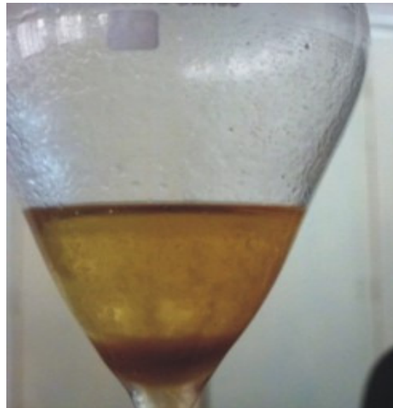
Plate 4c: Crude biodiesel and glycerol
