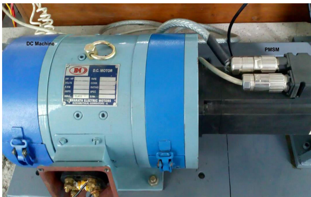
Fig. 3.31 Mechanically coupled PMSM and DC machine
