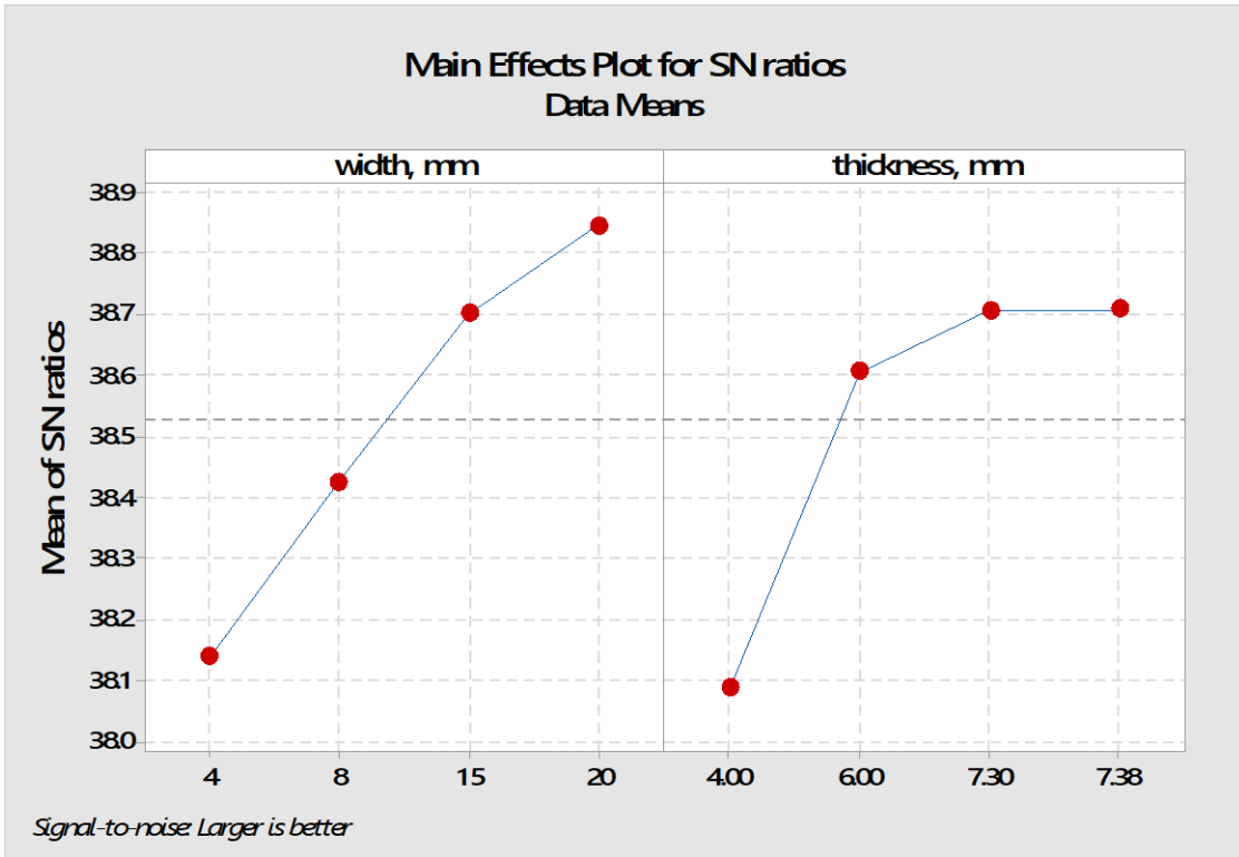
Fig. 4.16 Effect of magnet dimension on average S/N ratio for PMSM efficiency
