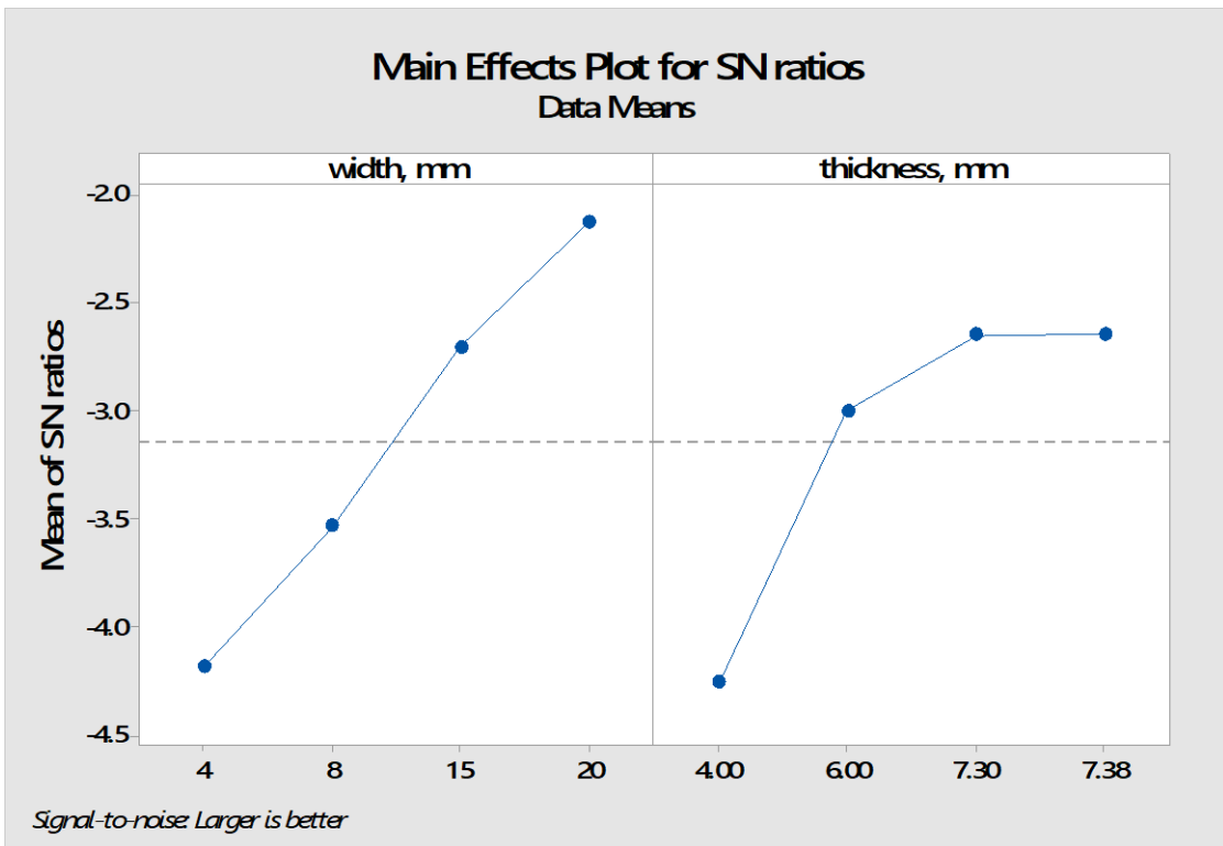
Fig. 4.17 Effect of magnet dimension on average S/N ratio for PMSM power factor
