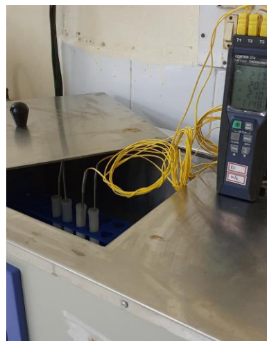
Fig. 3.4b Temperature control during thermal conductivity measurement of PCM
