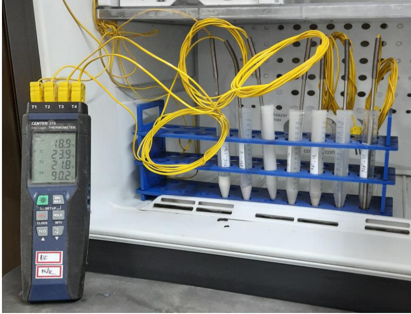
Fig. 3.20 Thermal Cyclic test of NePCM
