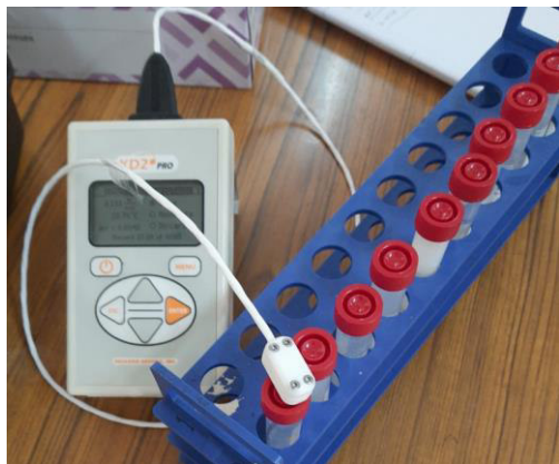
Fig. 3.4a Thermal conductivity measurement using KD2-pro thermal property analyzer
