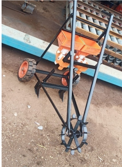
Fig. 3.12 Developed manual operated double row vegetable seed planter
