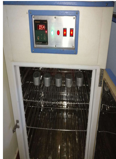
Fig.3.15 Determination of moisture content by oven drying method
