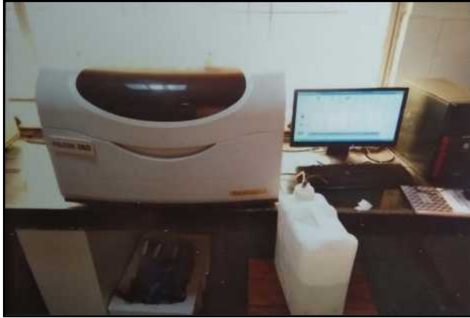
Plate no. 4.9 : Serum auto analyzer FALCON- 260.
