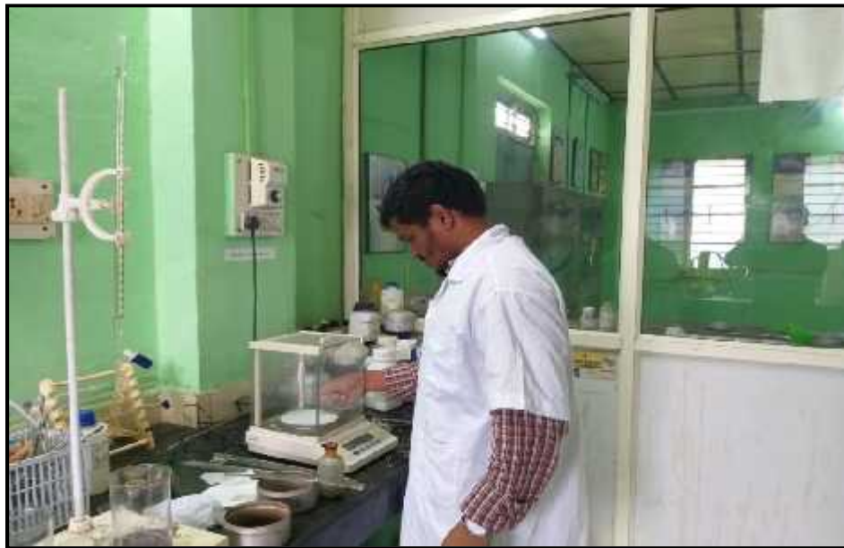
Plate no. 4.2: Weighing of feed sample for estimation of Ether Extract.
