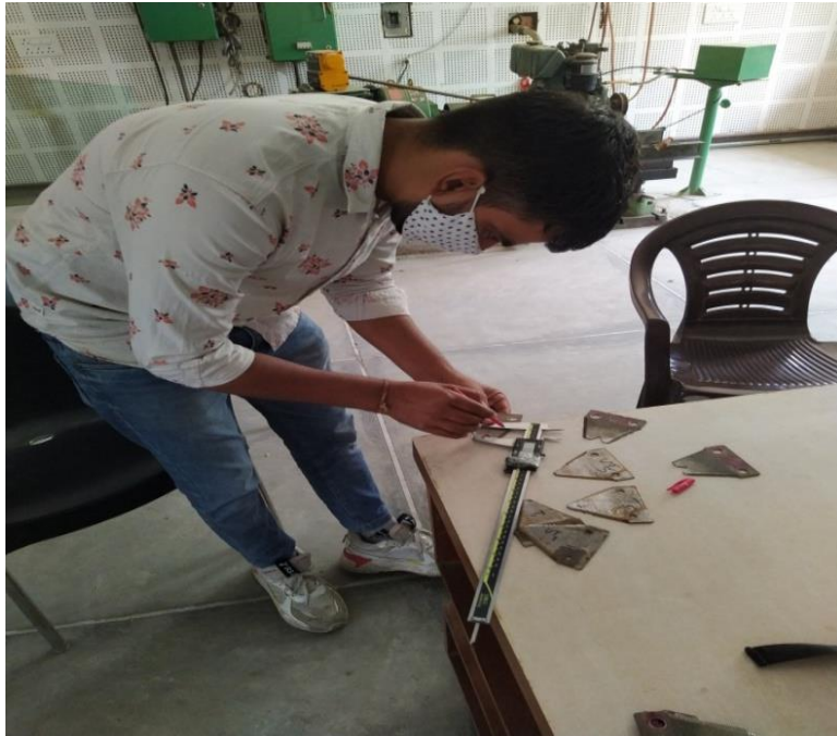
Fig. 3.17: Measurement of dimensions of blades (A and M type)
