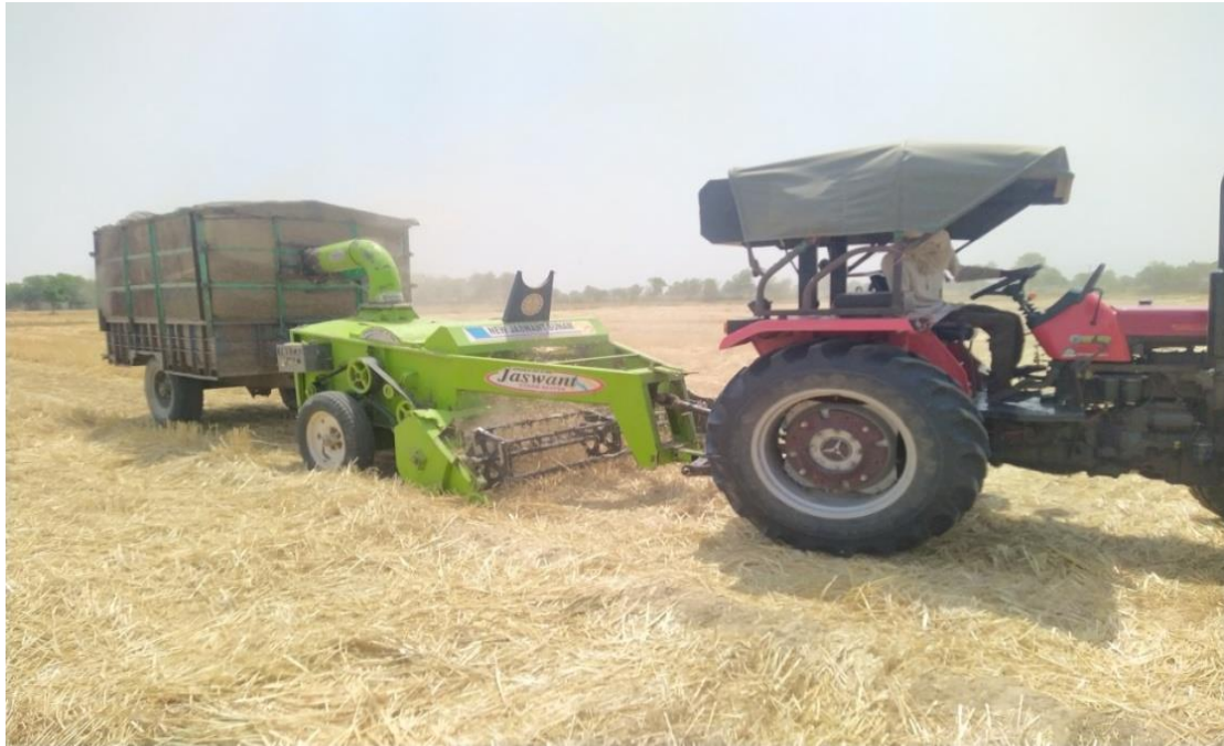
Fig. 3.14: Straw combine machine in operation in the field
