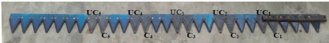
Fig. 3.12: Position of coated and uncoated blades on cutter bar (A type)
