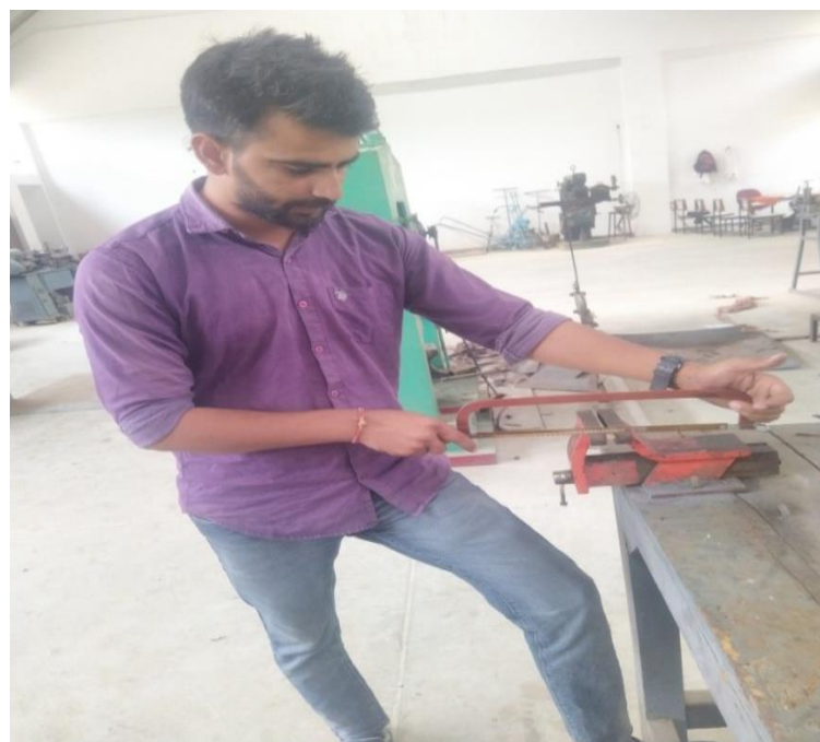
Fig. 3.2: Cutting of high carbon steel rod
