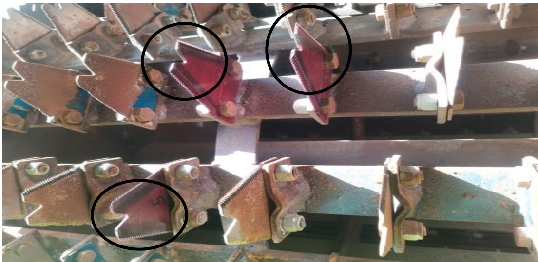
Fig. 3.13: Position of coated and uncoated blades (M type) in chopping cylinder
