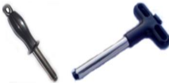
Fig 2.1: Tender coconut opener
