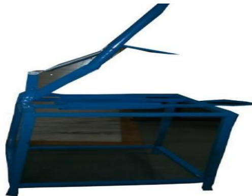
Fig 3.2: A hand operated model of tender coconut cutting machine
