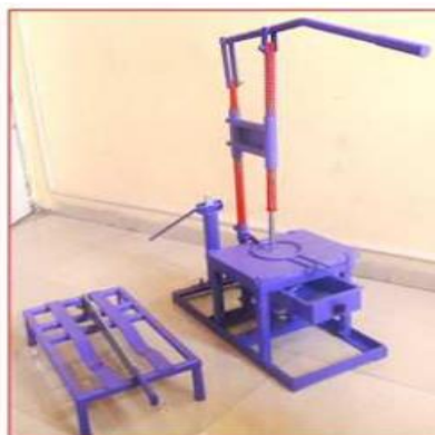
Fig 3.3: Multipurpose standing and sitting model of coconut cutting machine
