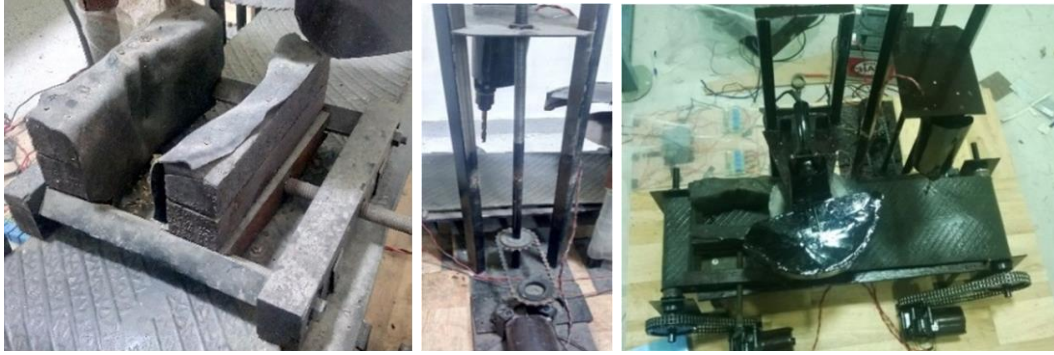
Fig. 4.2 Coconut chopping machine a) Coconut holder b) Drill mechanism c) Final assembled machine.
