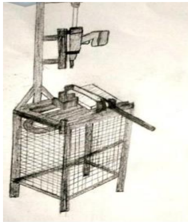
Fig 2.5: Mechanical facilitator for punching and splitting of tender coconut
