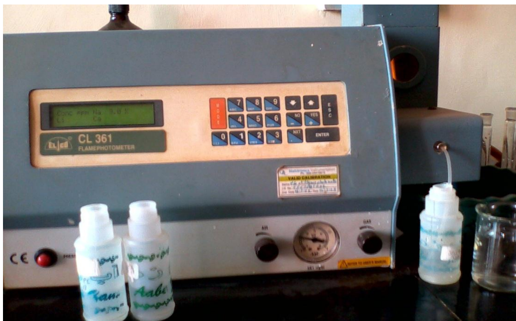
Fig. 3.20 Determination of Sodium by Flame Photo meter
