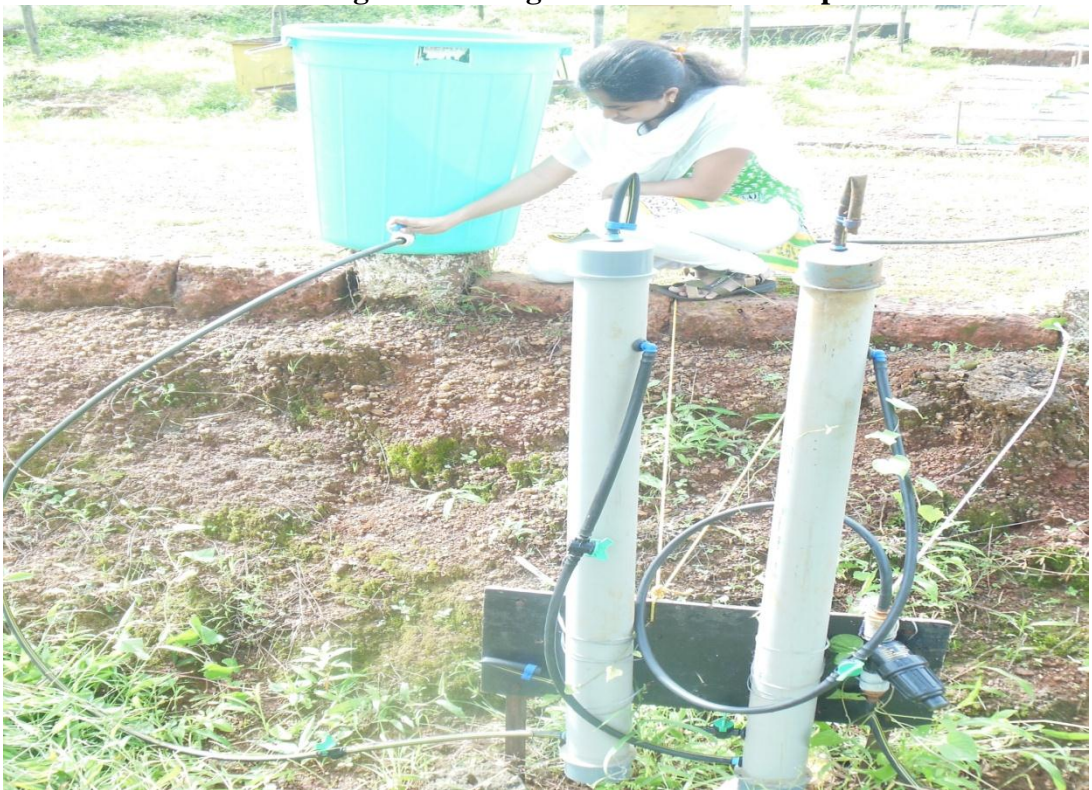
Fig. 4.16 Starting manual control valve
