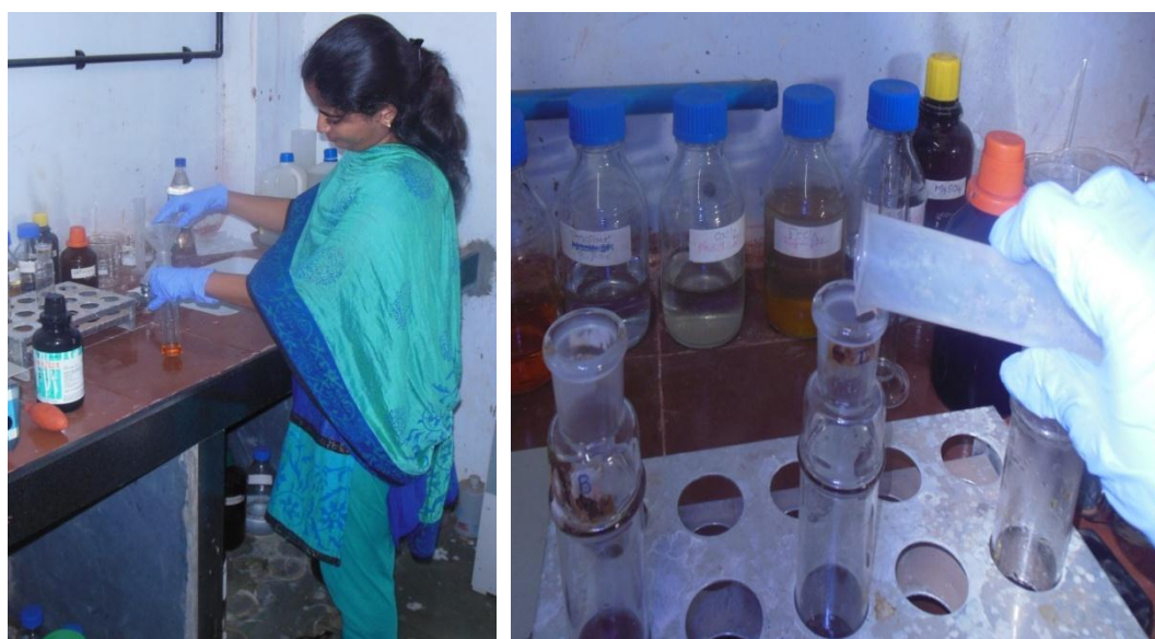
Fig. 3.23 Preparation of solutions for COD test
