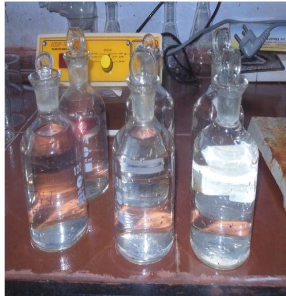
Fig. 3.26 BOD bottles for blank, inlet and outlet
