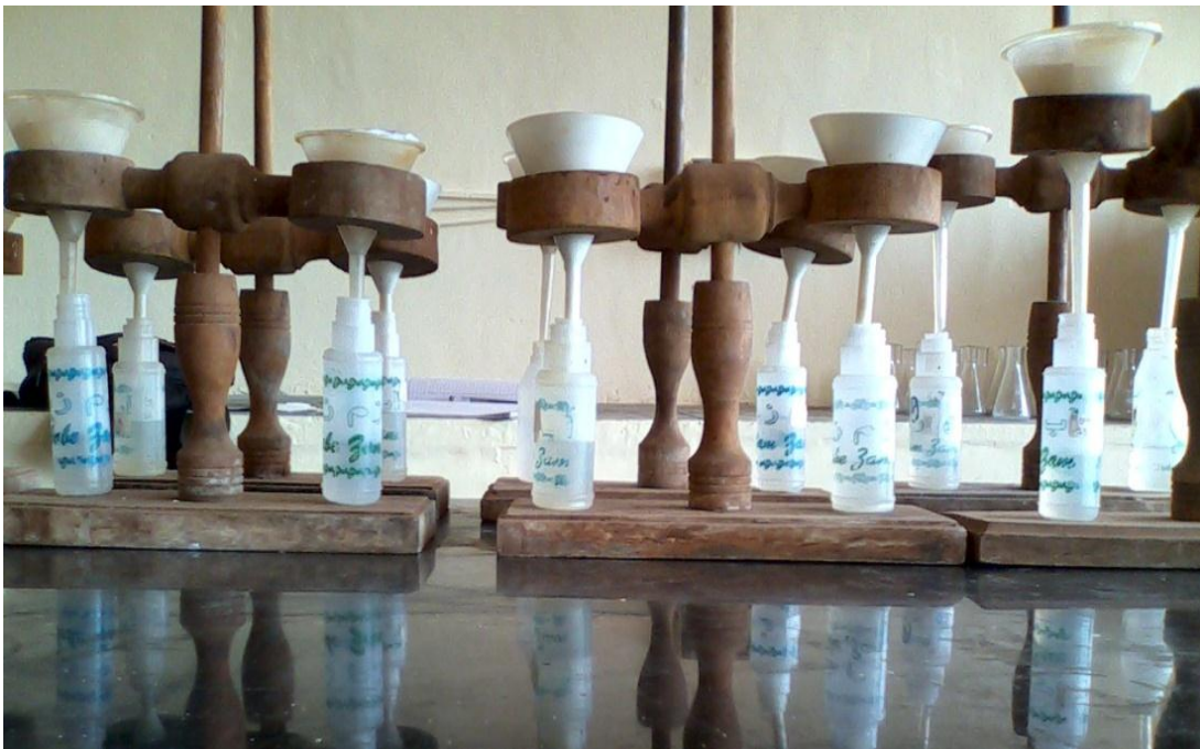
Fig. 3.19 Filtration of grey water sample by what man filter paper
