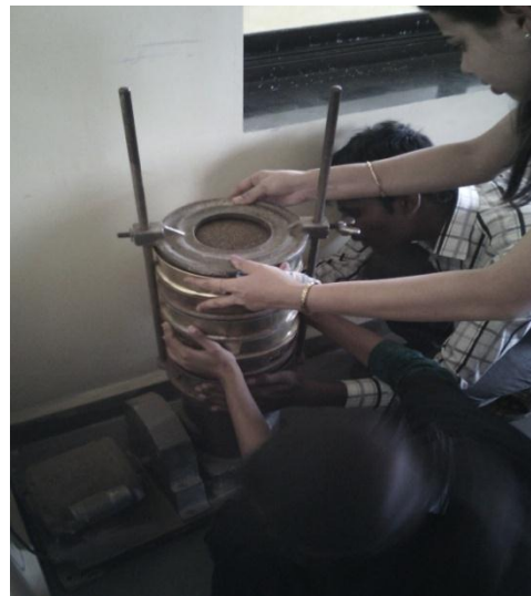
Fig. 3.10 Arrangement of sieves
