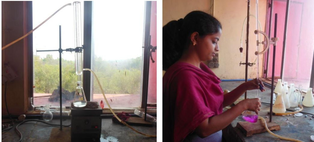
Fig. 3.22 Determination of oil and grease in grey water sample
