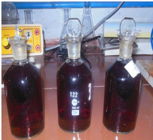
Fig. 3.29 PPT dissolve after adding H_2SO_4 solution Fig. 3.30 Solution after adding starch
