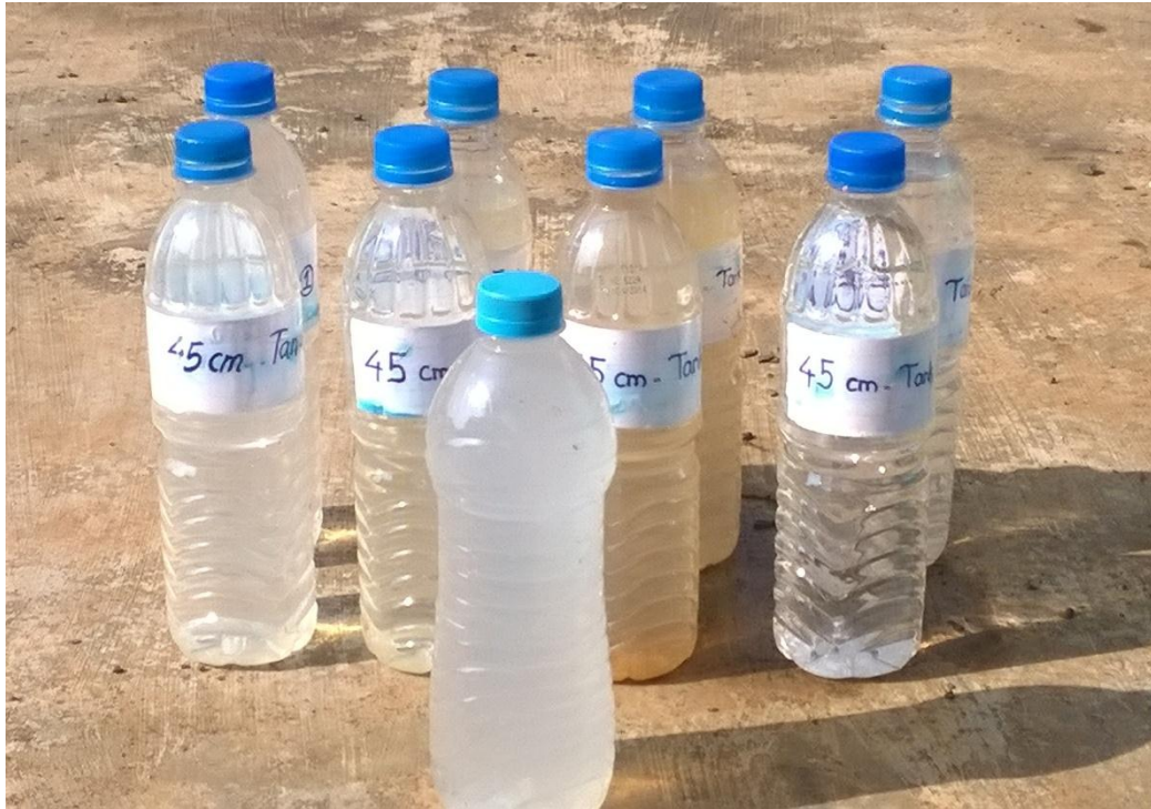
Fig. 3.14 Grey water after filtration at 45 and 15 cm depth
