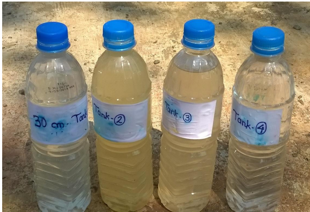
Fig. 3.13 Grey water after filtration at 30 cm depth
