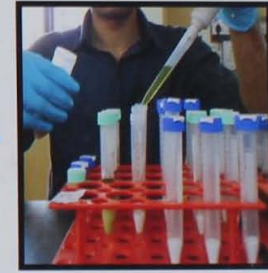
Drawing aliquot of 6 mL in 300 mg PSA and 900 mg MgSO 4
