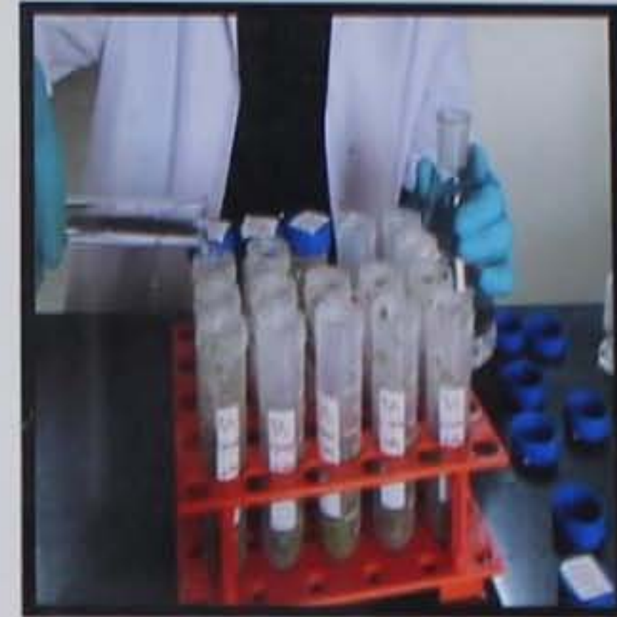
Addition of 15 mL 1% acetic acid in acetonitrile
