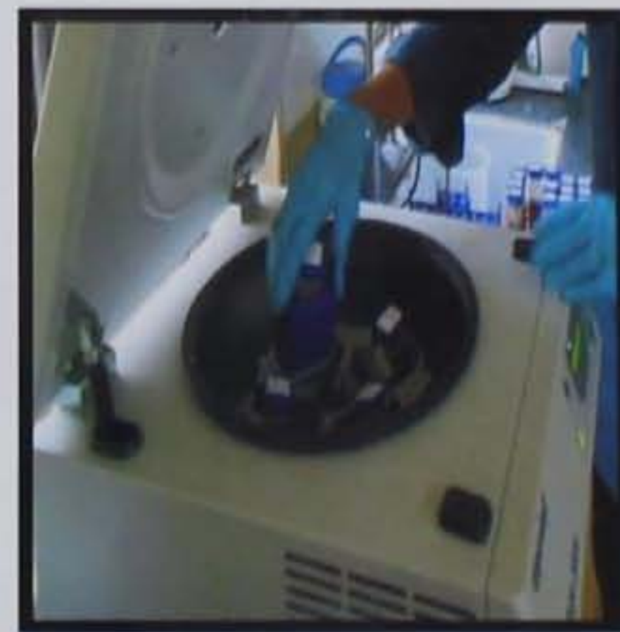
Centrifuge for 1 min at 3500 rpm
