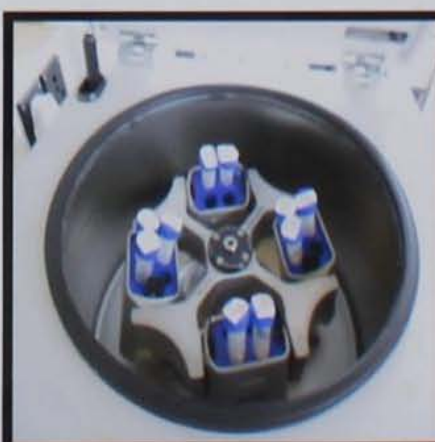
Centrifuge for 1 min at 2500 rpm
