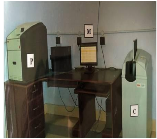
A. Conventional X ray machine with computerized radiographic unit [Printer(P), Monitor(M), Console(C)]
