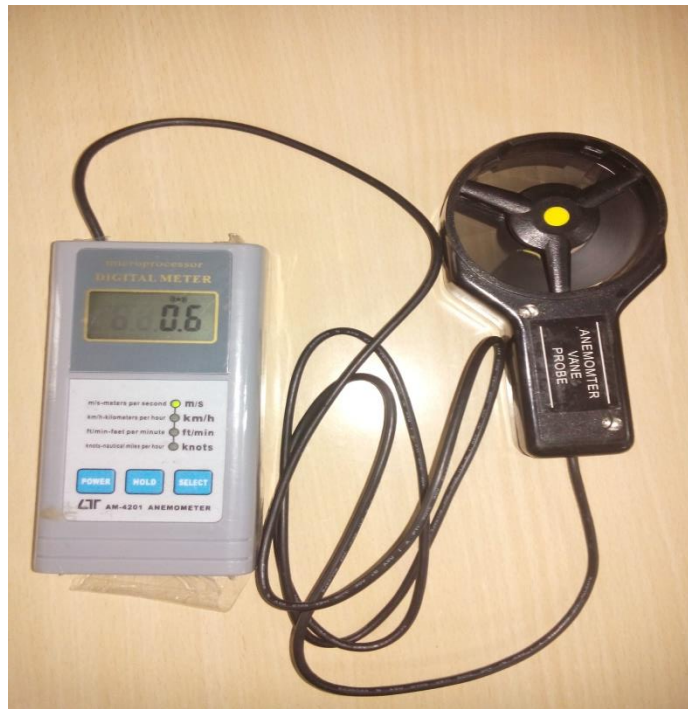
Fig. 3.16 Schematic diagram of anemometer
