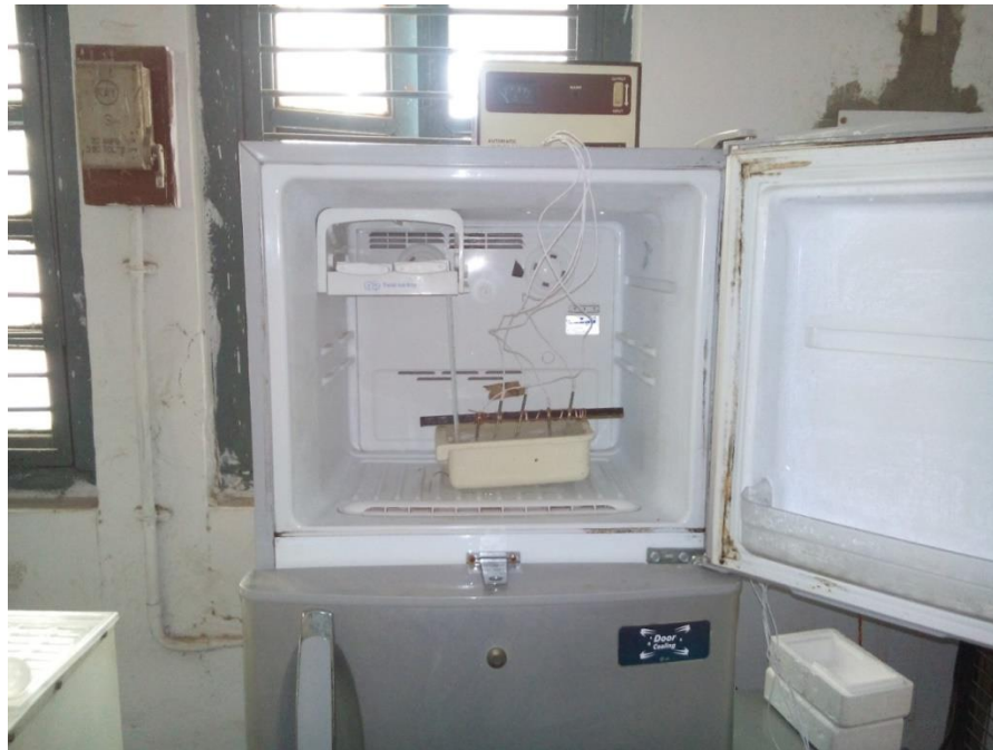
Fig. 3.14 Schematic diagram of calibration of data logger
