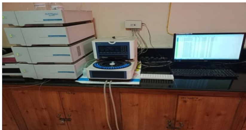
Fig. 3.2 HPLC system used for herbicide extraction
