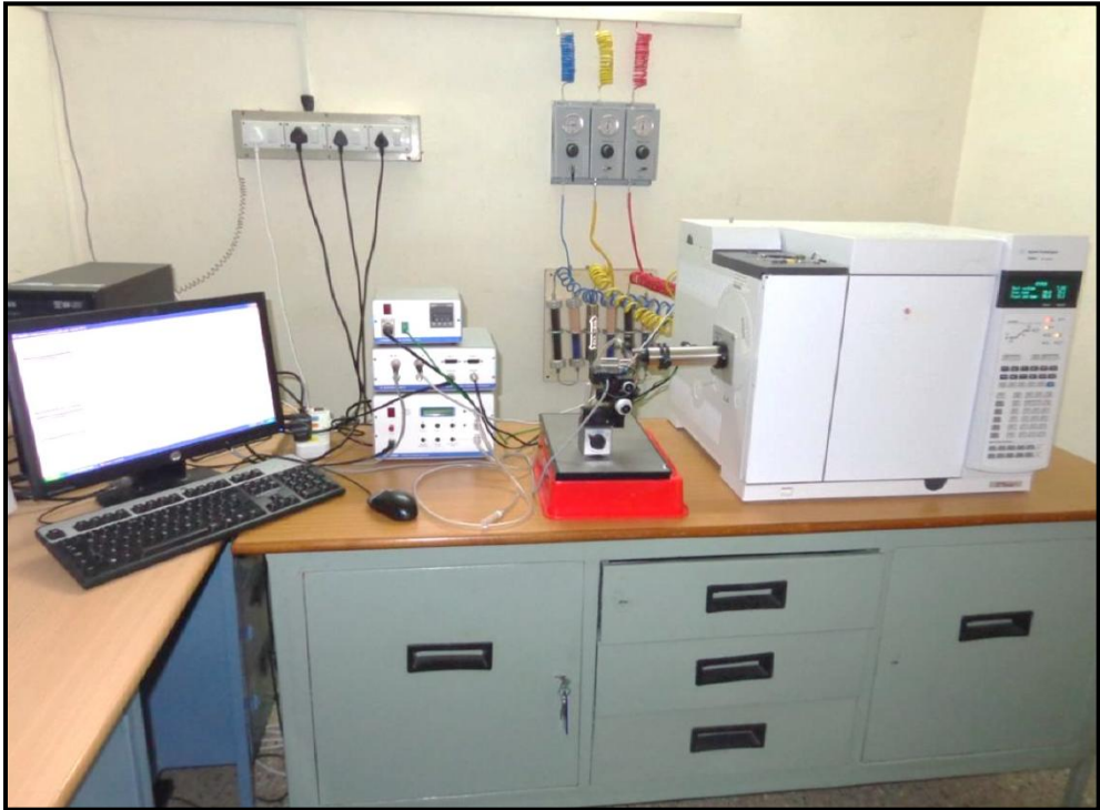
Plate 4. Coupled gas chromatography-electro antennogram detector (GC-EAD) instrument
