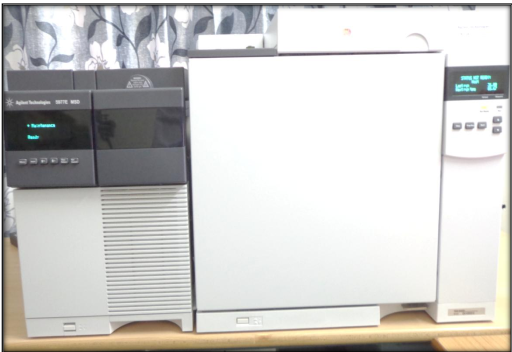
Plate 5. Coupled gas chromatography-mass spectrometry (GC-MS) instrument
