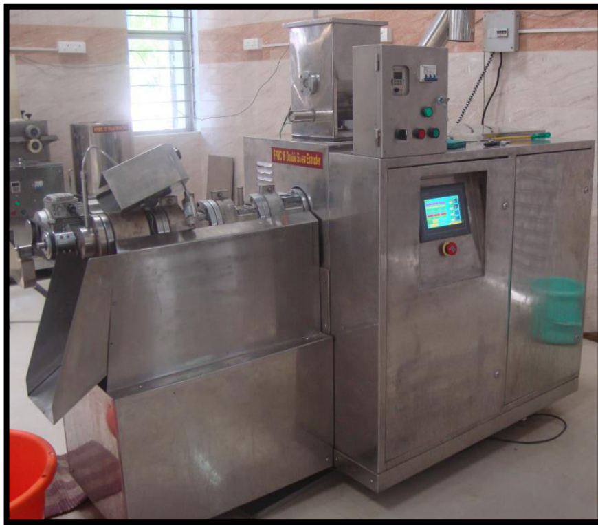
Plate: 3.5 Co-Rotating Twin-Screw Extruder
