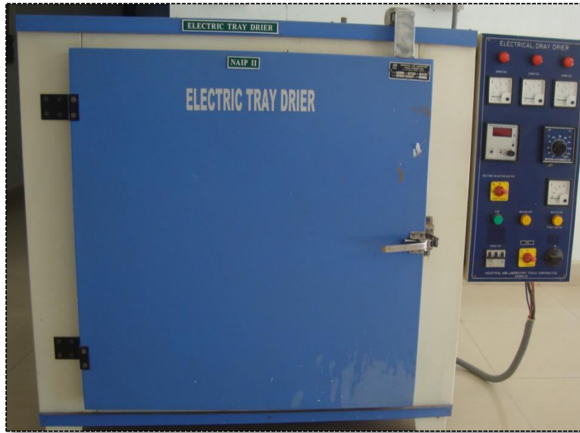
Plate: 3.1 Forced – Electric Tray drier
