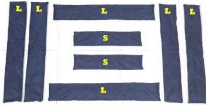
Fig. 12: Fabricated sandbags using PVC American Matty
