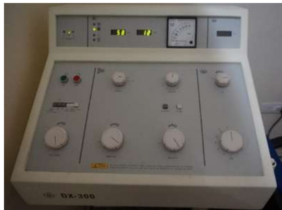
Fig. 3: Control panel of the X-ray machine (Wipro GE DX-300) showing exposure settings of 50 kVp and 12 mAs
