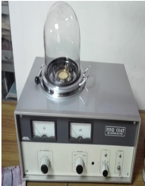
(a) Ion sputter coater machine (model Jeol JFC-1100, USA)
