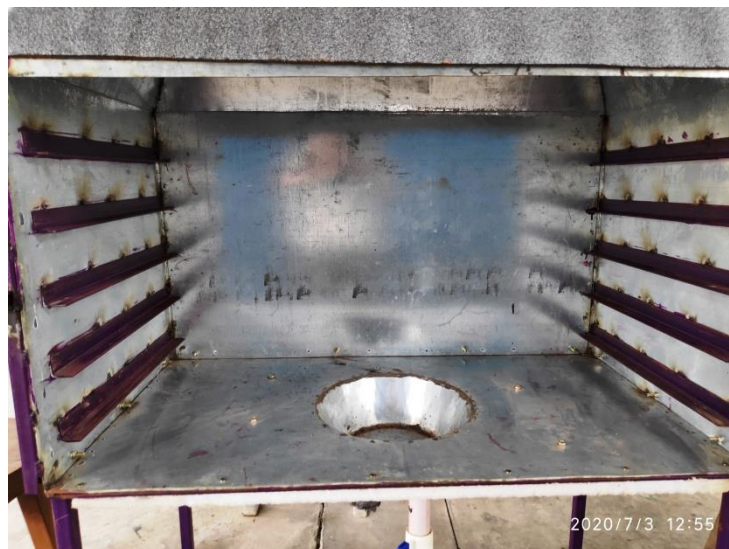
Plate 3.1 Inside view of drying chamber
