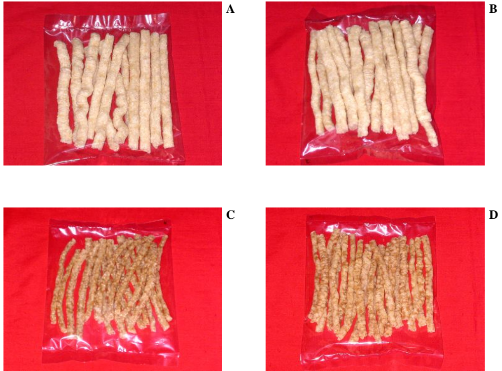
Fig. 26: Extruded products from wheat semolina-ribbonfish mince mixture A: with 10% ribbonfish mince at 70°C B: with 10% ribbonfish mince at 90°C C: with 20% ribbonfish mince at 70°C D: with 20% ribbonfish mince at 90°C (Products prepared at a screw speed of 350 RPM using 4 mm die diameter)
