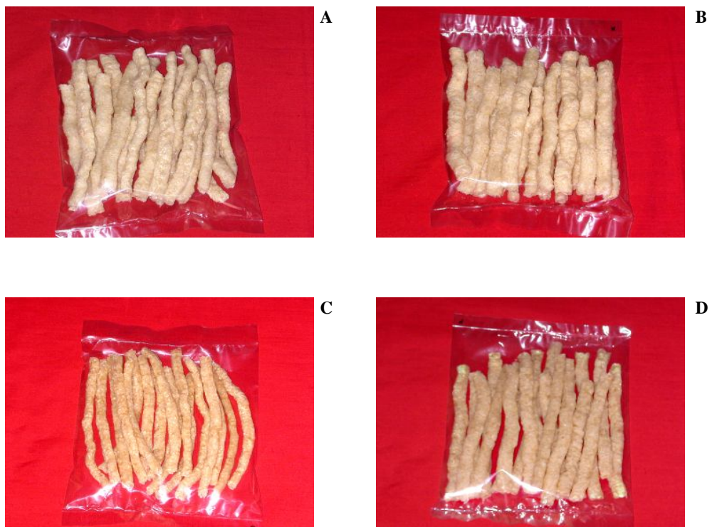
Fig. 27: Extruded products from wheat semolina bull's eye fish mince mixture A: with 10% bull's eye mince at 70°C B: with 10% bull's eye mince at 90°C C: with 20% bull's eye mince at 70°C D: with 20% bull's eye mince at 90°C (Products prepared at a screw speed of 350 RPM using 4 mm die diameter)
