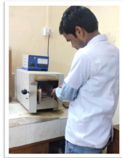
Determination of Ash
