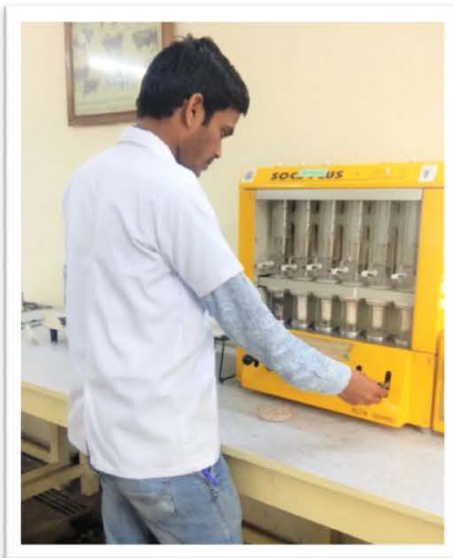
Determination of ether extract
