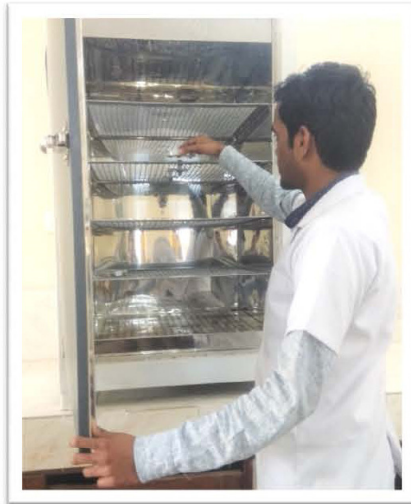
Determination of dry matter
