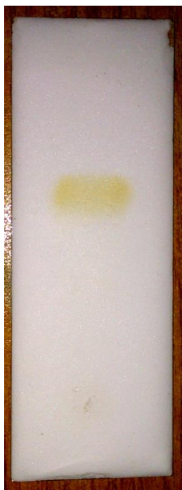
Thin layer Chromatography of Scytonematopsis strain extracts with one band designated as A1.
