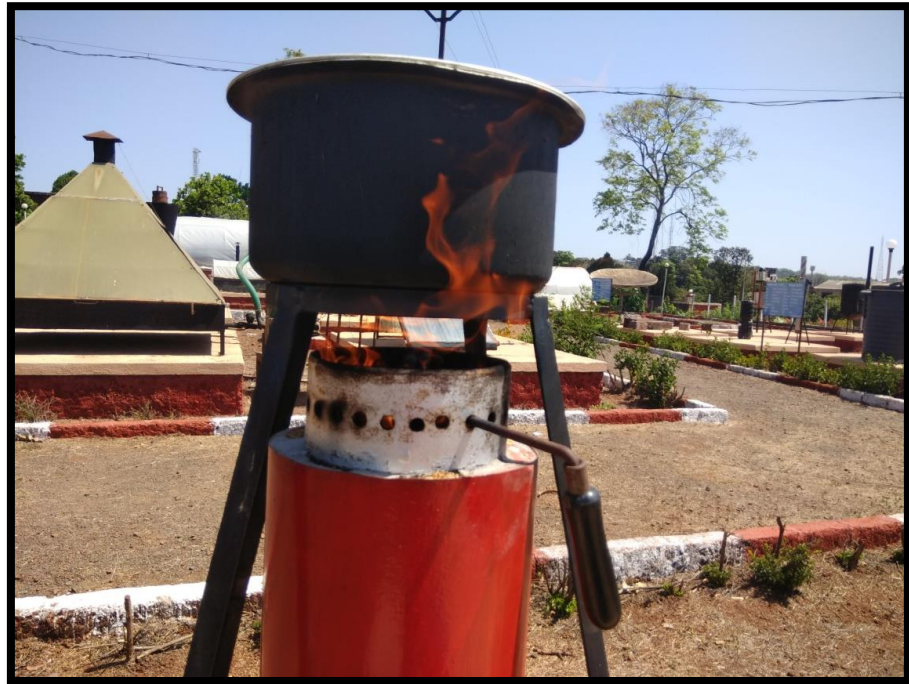
Plate-3.6 Standard water boiling test during laboratory testing of rice husk based gasifier.
