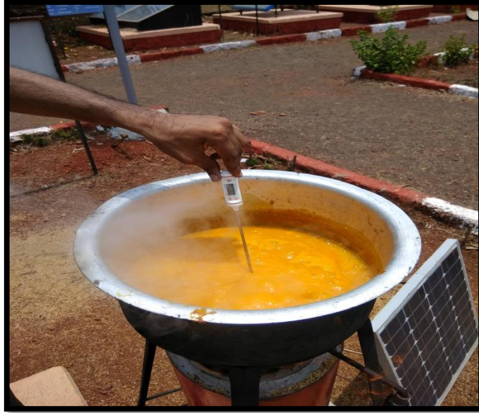
Plate-3.8 Mango pulp boiling during field testing of rice husk based gasifier.
