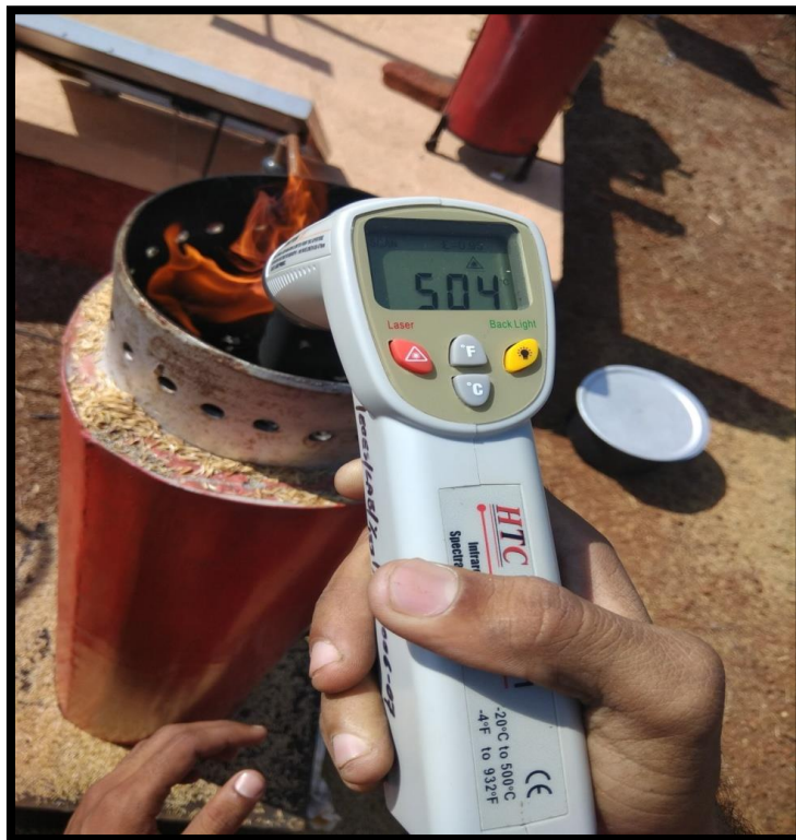
Plate-3.7 Thermal profile test during laboratory testing of rice husk based gasifier.
