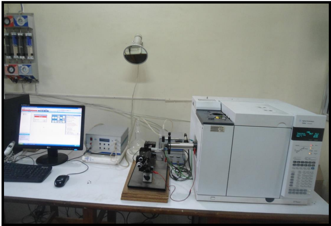
Plate 9. Electrophysiology Coupled Gas Chromatography - Electroantennodetector
