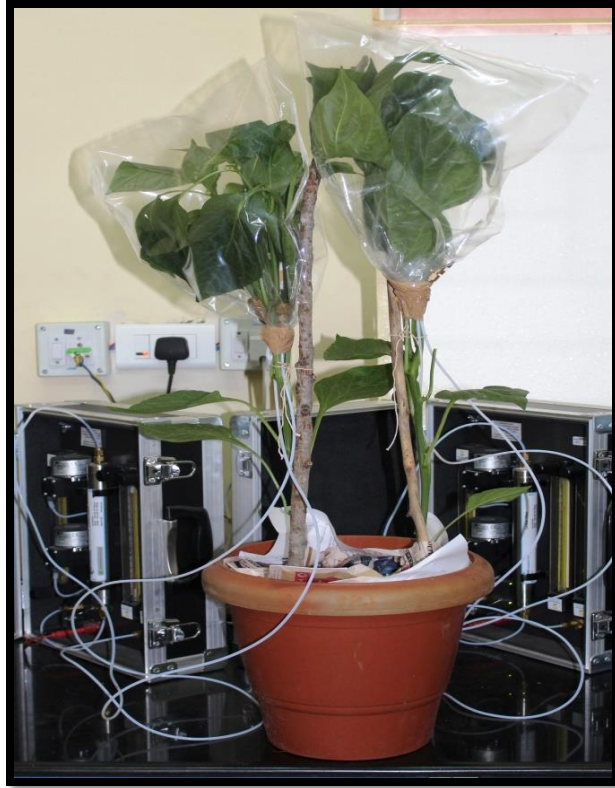
Plate 4. Collection of host plant headspace volatiles using air entrainment system
