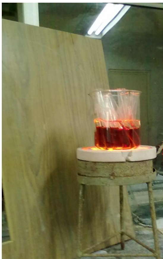
Determination of total organic matter by Scholenberger method
