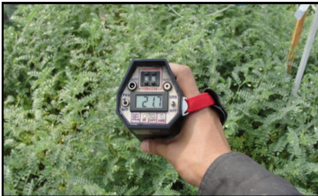
Determination of canopy temperature by IR thermometry
