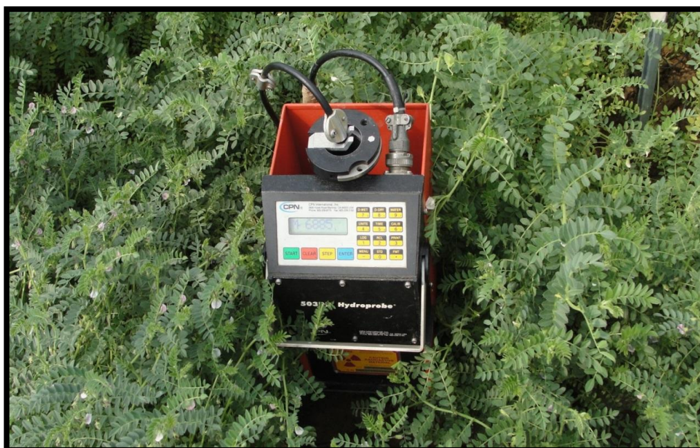
Determination of crop water use by neutron moisture meter (Soil moisture depletion method)
