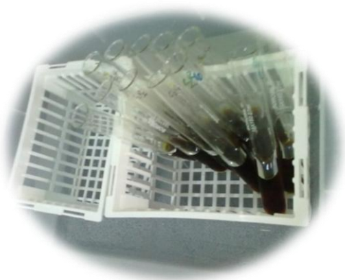
Determination of total organic matter by Scholenberger method
