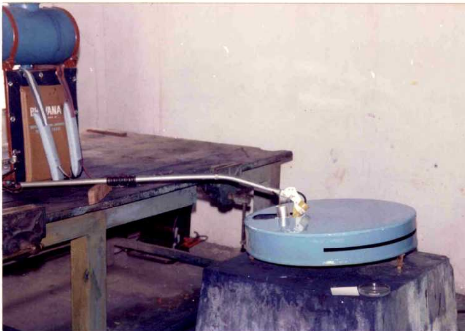
Plate 2. Spread factor determination with narrow spectrum droplet generator
