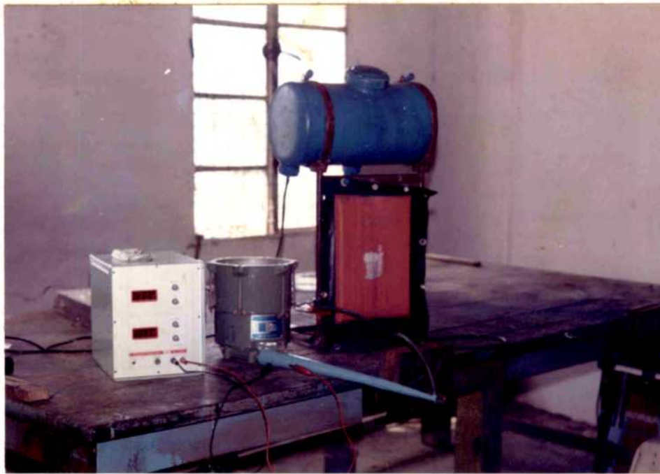
Plate 7. DC motor operated pneumatic spraying system
