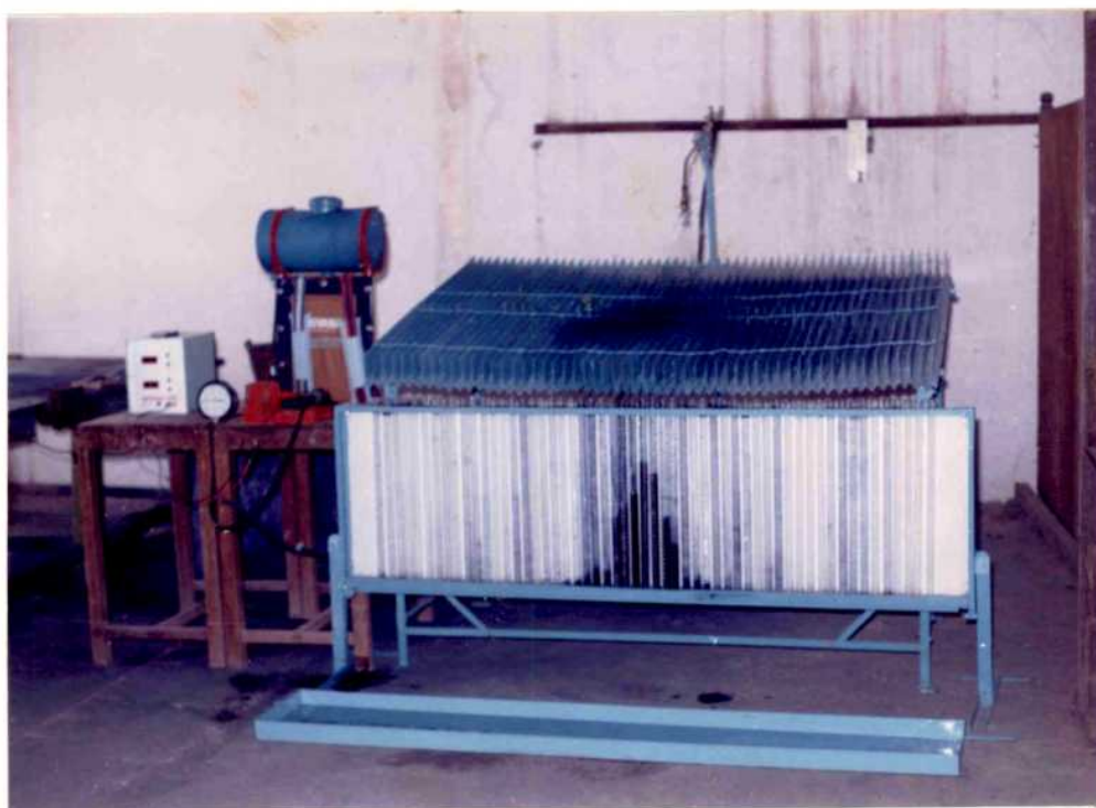
Plate 6. Spray distribution pattern of DC motor operated hydraulic spraying system
