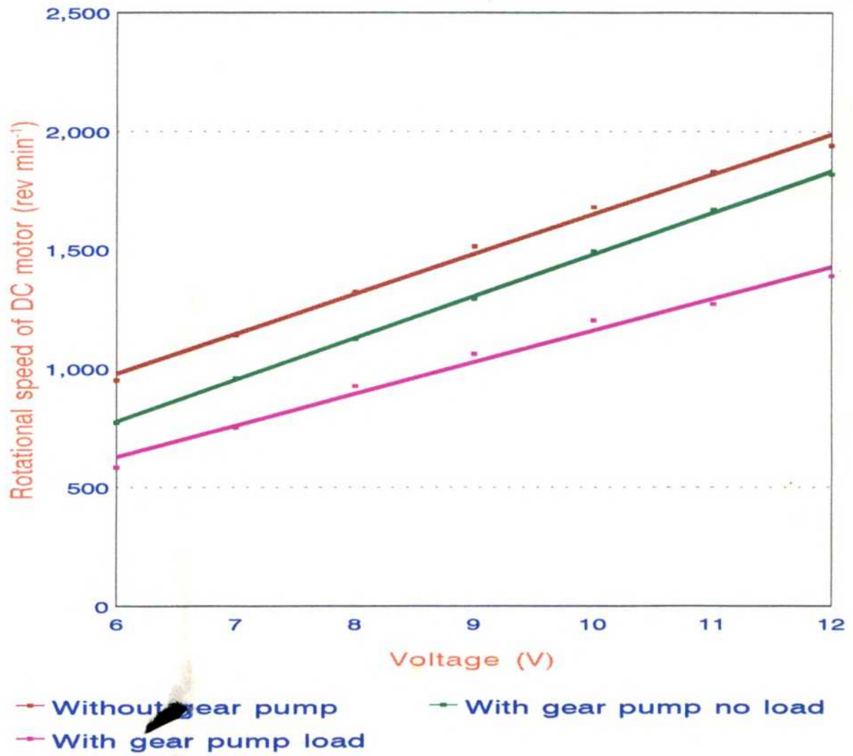
Fig. 4.4 Rotational speed of DC motor at varying voltage
