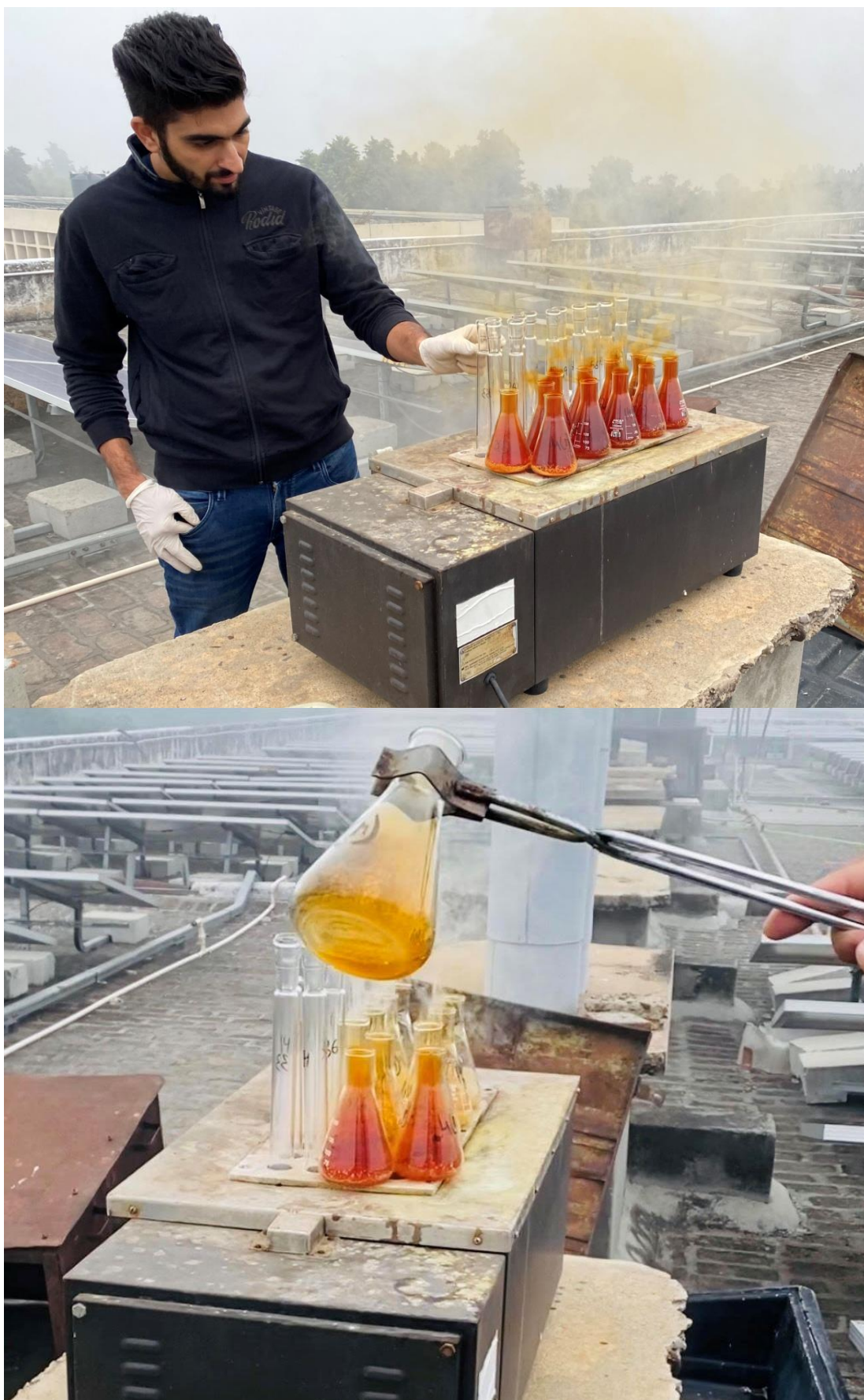
Plate 4: Digestion of samples for mineral analysis
