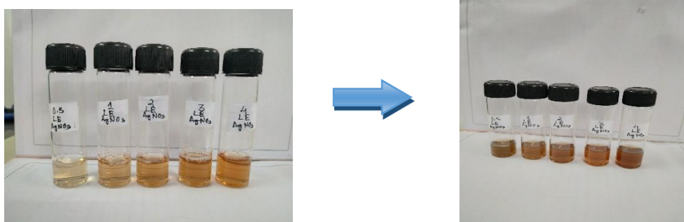
Fig 7: color change indicating the synthesis of silver nanoparticles
