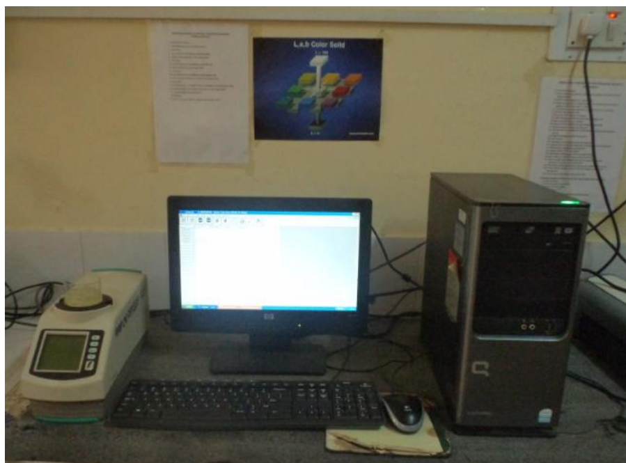
Plate 8. Hunter lab Colourimeter used for measuring the colour values of Aloe vera gel
