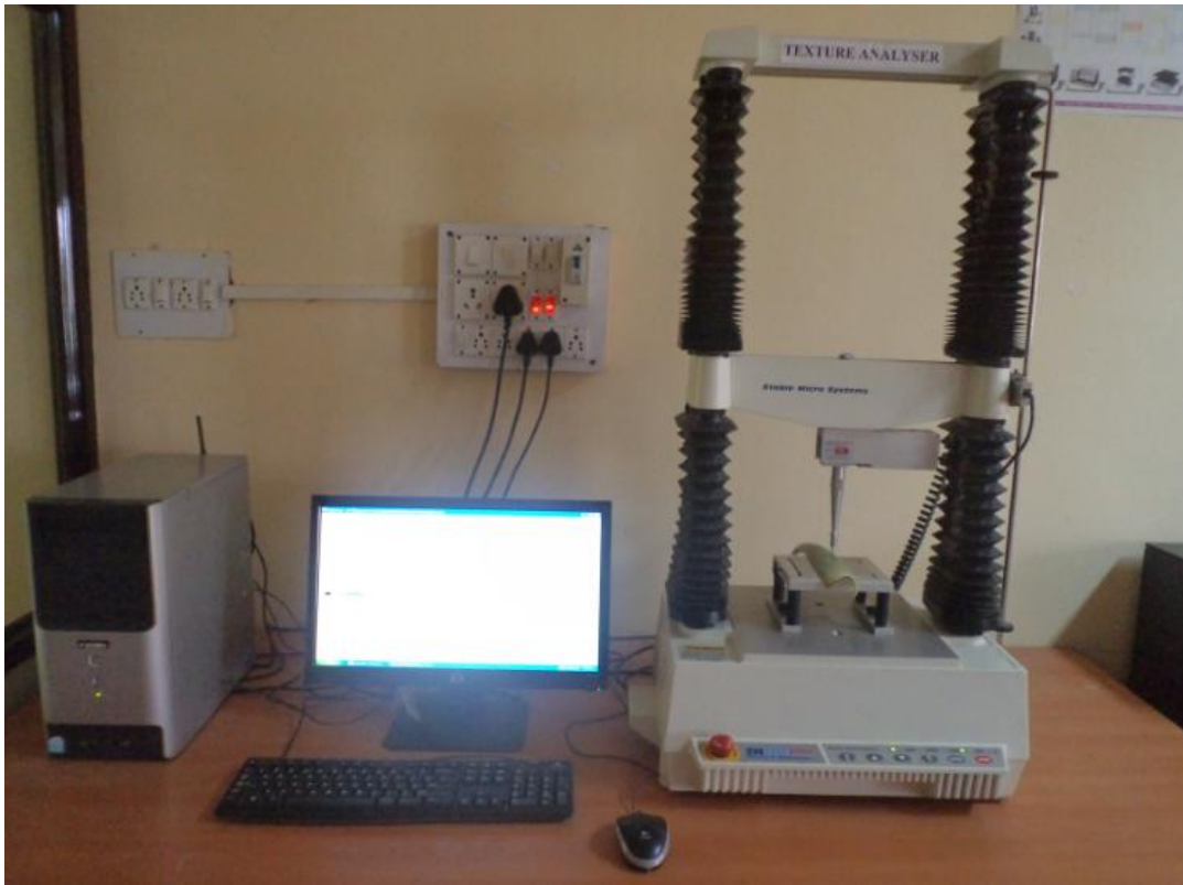
Plate 1. Texture analyser used for measuring the firmness of Aloe vera leaf
