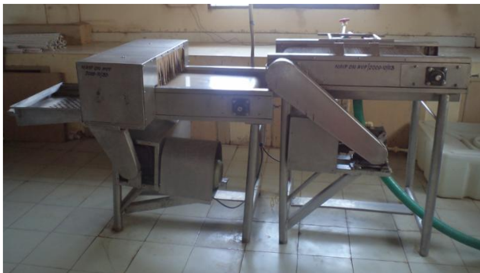
Plate 4. Aloe vera gel extraction machine combined with Aloe vera leaf washing machine
