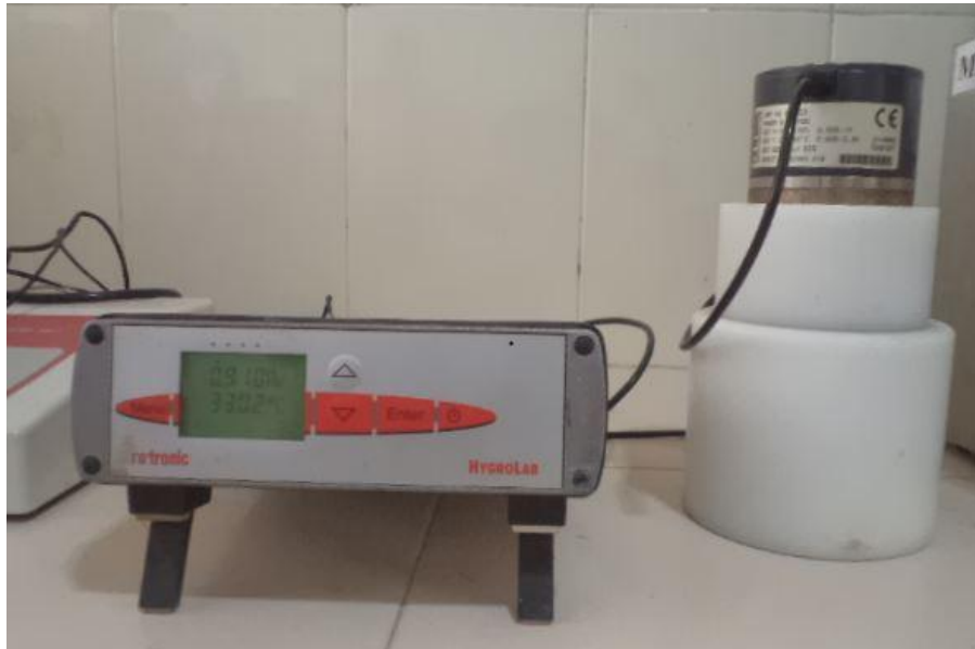
Plate 7. Water activity meter used for measuring the water activity of Aloe vera gel
