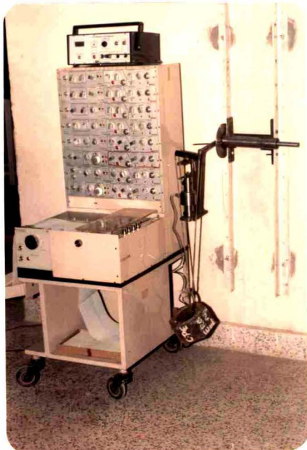
Fig. 4.10 Calibration of load cell using dead load
