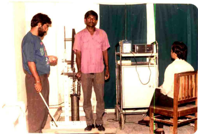
Fig. 4.7 Experiment-2 for optimization of frequency of handle operation- Measurement of heart rate
