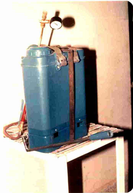
Fig. 4.14 (a) Modified sprayer mounted on test rig Fig. 4.14 (b) Measurement of number of strokes/min required to maintain 3 (\pm 10 \text{ per cent}) \text{kg/cm}^2 pressure Fig. 4.14 (c) Measurement of discharge at 3 (\pm 10 \text{ per cent}) \text{kg/cm}^2 nozzle pressure for one minute Fig. 4.14 Preliminary trials of modified sprayers unit
