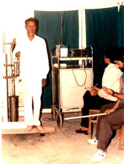
Fig. 4.3 Experiment-1 for determination of optimum frequency and range of handle movement-Measurement of heart rate
