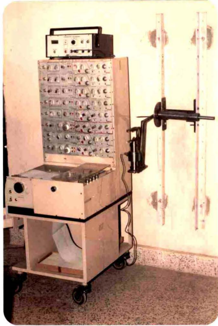
Fig. 4.9 (b) Setup along with polyrite recorder unit for measurement of muscular strength
