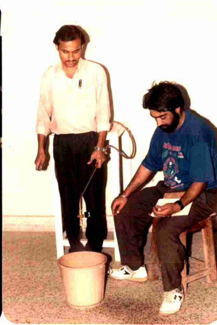
Fig. 4.14 (a) Modified sprayer mounted on test rig Fig. 4.14 (b) Measurement of number of strokes/min required to maintain 3 (\pm 10 \text{ per cent}) \text{kg/cm}^2 pressure Fig. 4.14 (c) Measurement of discharge at 3 (\pm 10 \text{ per cent}) \text{kg/cm}^2 nozzle pressure for one minute Fig. 4.14 Preliminary trials of modified sprayers unit
