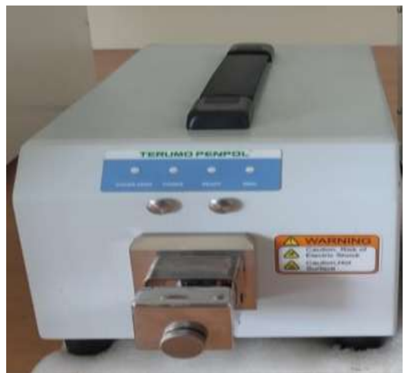
Plate 6e: Tube sealer used to permanently close a fluid path and creation of pig tails for compatibility testing
