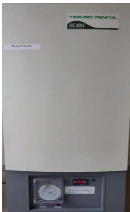
Plate 6g: Deep freezer -40 °C used for the storage of fresh frozen plasma
