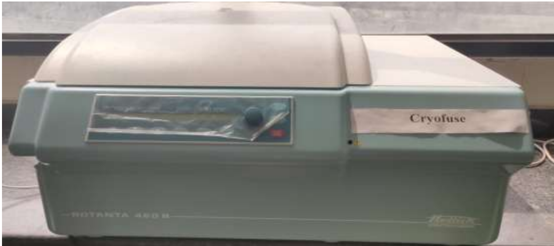
Plate 6a: Temperature controlled centrifuge (Cryofuse) used to process whole- blood derived products
