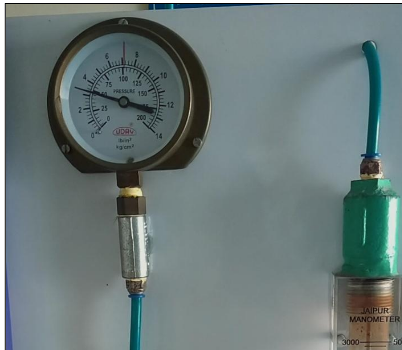
Fig.3.10 Pressure gauge provided in patternator
