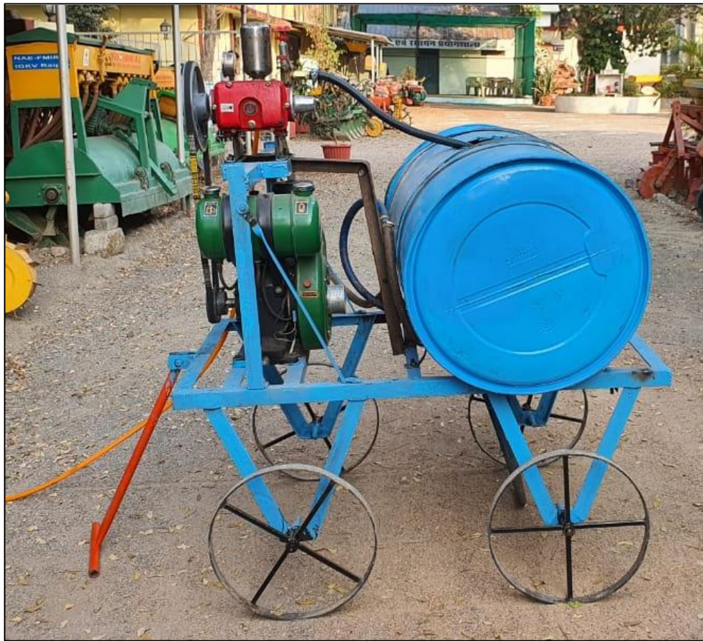
Fig 3.15 Actual view of chemical storage cum power unit
