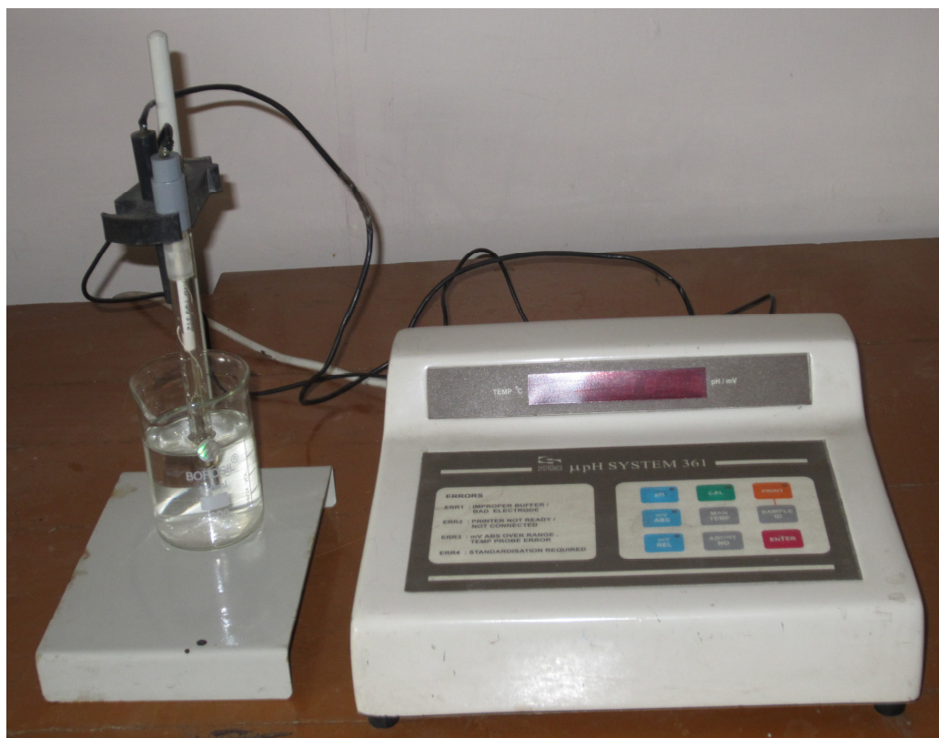
Figure 3.4 pH meter showing the pH probe and mercury thermometer
