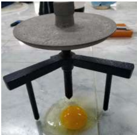
Figure-8: Measuring the thick albumen height with spherometer
