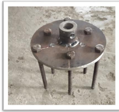
Plate 3.8 Rotating disc with cutting spikes (2, 4 and 6) Fig3.3 CAD view of rotating disc
