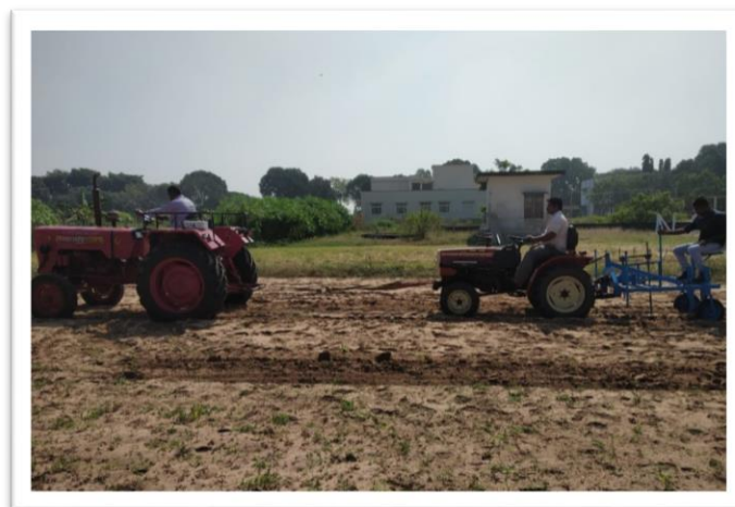
Plate 3.18 Measurement of draft in the field
