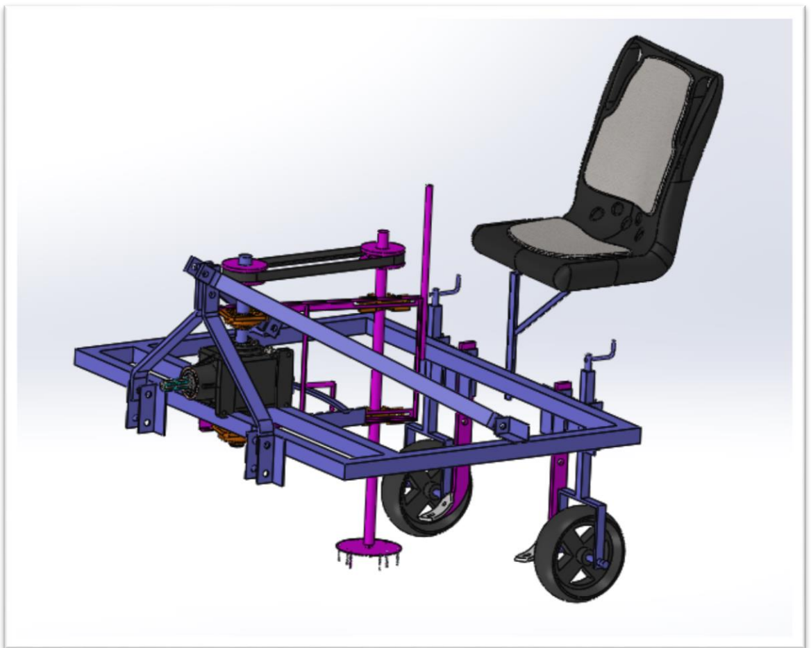
Fig. 3.5 – CAD representation of prototype (isometric view)
