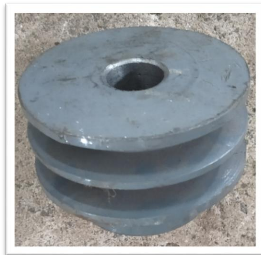
Plate 3.7 Pulley (101mm dia)
