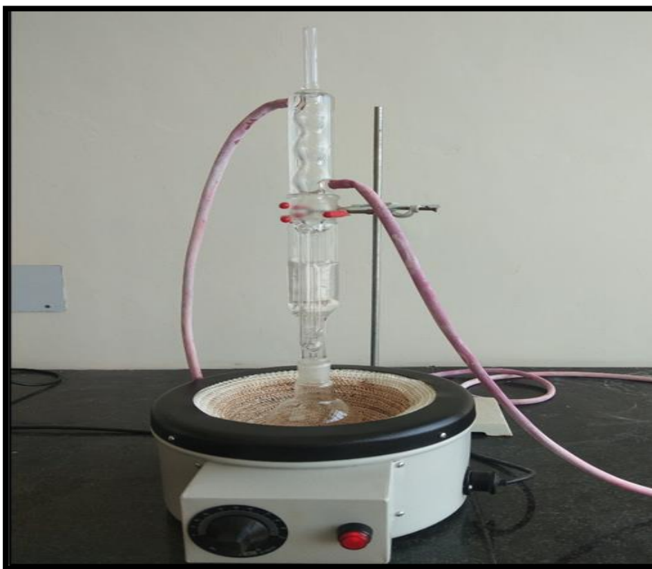
Plate 8. Extraction of oil using Soxhlet apparatus
