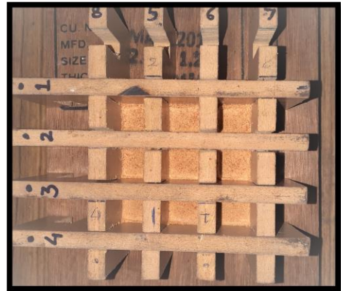
Plate 3.6: Compressed jaggery powder
