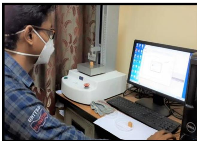
Plate 3.22: Textural analysis of jaggery cubes
