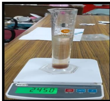
Plate 3.21: True volume analysis of jaggery cubes
