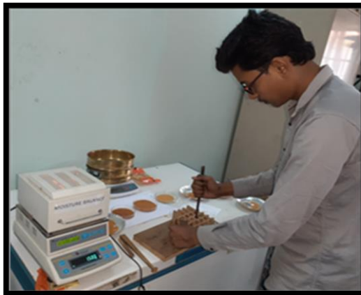
Plate 3.5: Compression of jaggery powder
