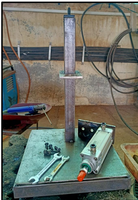
Plate 3.5 Fabrication of cutting mechanism mounting stand
