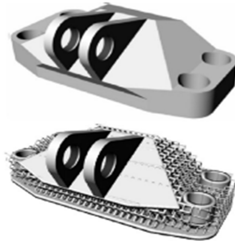
Figure. 2.1 An engine bracket in filled with strut-based lattice (Tang et al. 2015)
