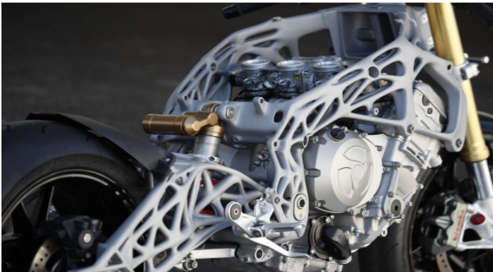
Figure. 1.2 Topology Optimized 3d Printed Frame (Abdi, Ashcroft and Wildman, 2018)
