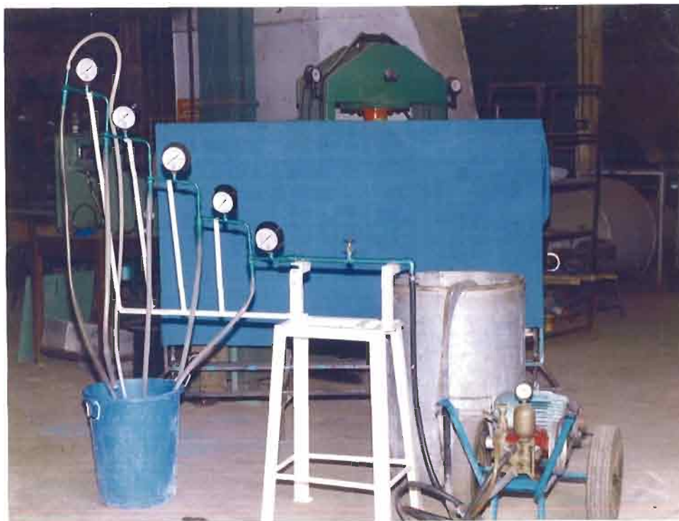
Plate. 3.7 Modified battery of hydro cyclones
