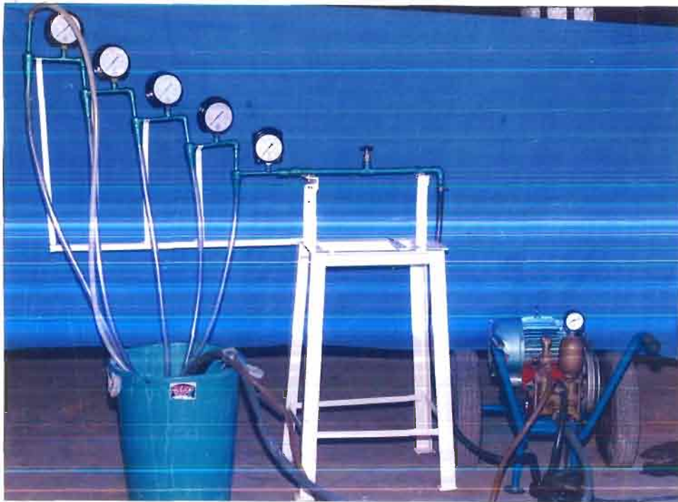
Plate. 3.6 Battery of hydro clones
