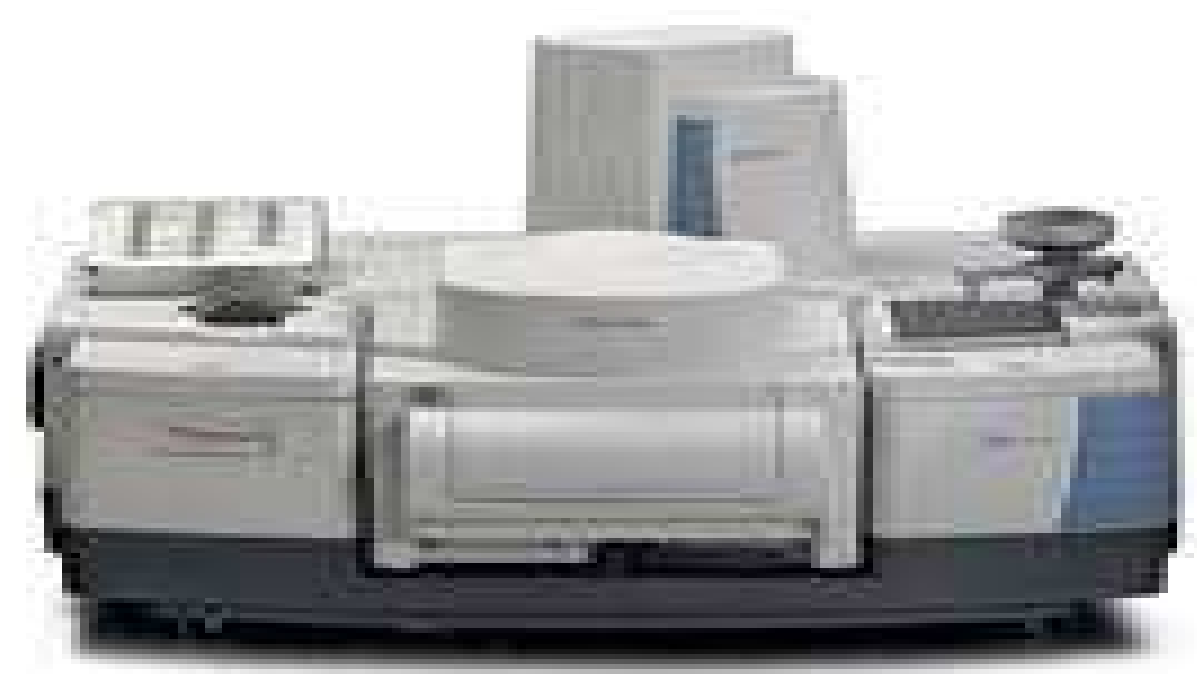
Figure 3.5 Photograph of Nicolet 6700 used for obtaining FTIR spectra
