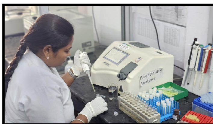
Pate 3.9. Analysis of biochemical Parameters (Total protein, Albumin and LDH enzyme) by using semi-automatic Biochemical analyzer
